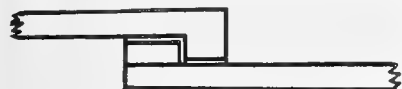
FIG. 153—LOCKING ENDS OF PORTABLE FENCE PANELS This drawing shows manner in which ends of portable fence panels are locked. Also see Fig. 155.
