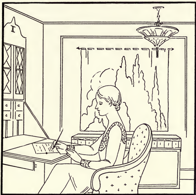
FIG. 4.—Illumination provided from an extended light source, the ceiling, similarly found out of doors on an overcast day, provides softness of shadow and eye comfort.
