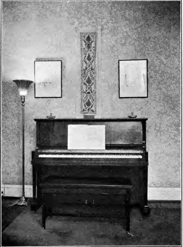
FIG. 33.—An indirect floor lamp fills the piano corner with even, shadowless light of which the sheet music receives its adequate share.
