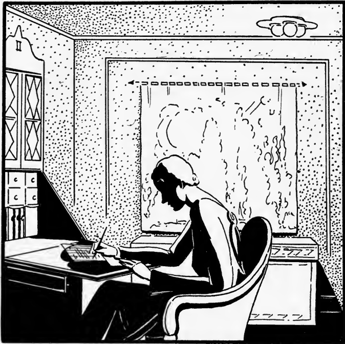
FIG. 3.—Illumination provided with unshaded lamp bulbs results in harsh shadows and impaired eye comfort. The size of the principal light source (the unshaded lamp bulbs) is too small.
