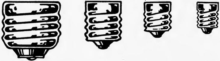
FIG. 6.—Lamp bases (actual size). 1. Medium screw base. 2. Intermediate screw base. 3. Candelabra screw base. 4. Miniature screw base.
