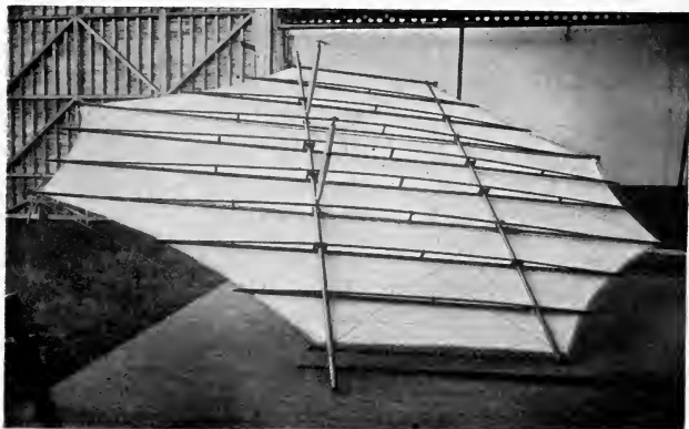
Fig. 76.—The forward rudder of my large machine, showing the fabric attached to the lower side. The top was also covered with fabric. This rudder considered as an aeroplane had a very high efficiency and worked very well indeed.
