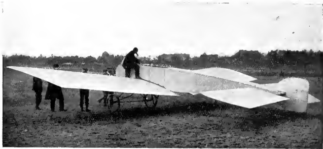
Fig. 71.—Bleriot's machine. This machine raised itself from the ground, but as the centre of gravity was very little, if any, above the centre of lifting effect, it turned completely over in the air.
