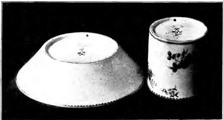
17. PÂTE TENDRE CUP AND SAUCER. Showing the Holes for Suspension in the Kiln. Sèvres, France, 1774. Bloomfield Moore Collection.
