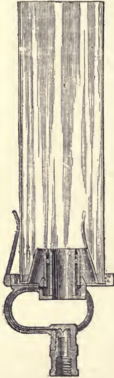
Fig. 20.—Section of Argand Gas Burner.
