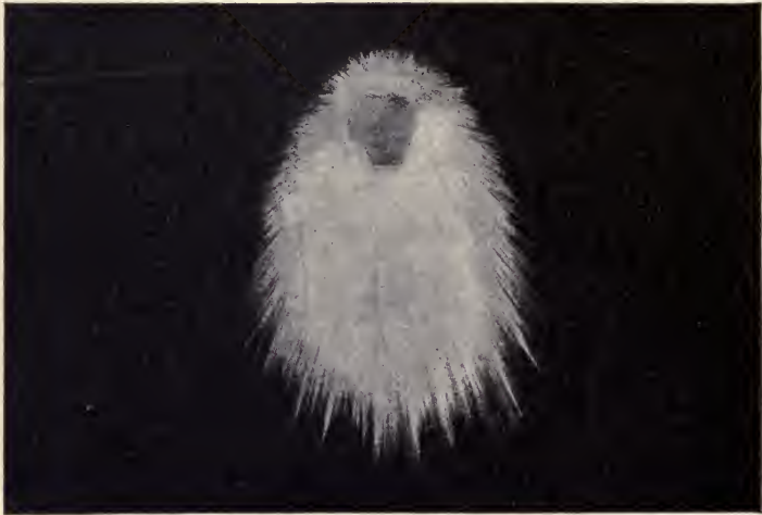
Fig. 74.—Holophane, Downward Distribution.
