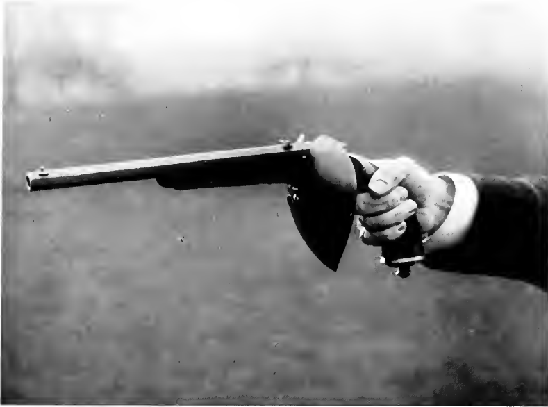
HOW TO HOLD THE DUELLING PISTOL WITH GUARD FOR SHOOTING DEVILLIER'S BULLET
