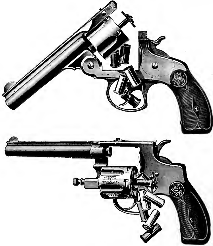
TWO SYSTEMS OF EJECTING SMITH & WESSON
