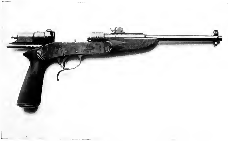
BELGIAN SINGLE-SHOT PISTOL.—SAW-HANDLE Showing breech open
