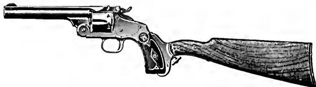
EXTENSION STOCK AS APPLIED TO .44 SINGLE-ACTION REVOLVER
