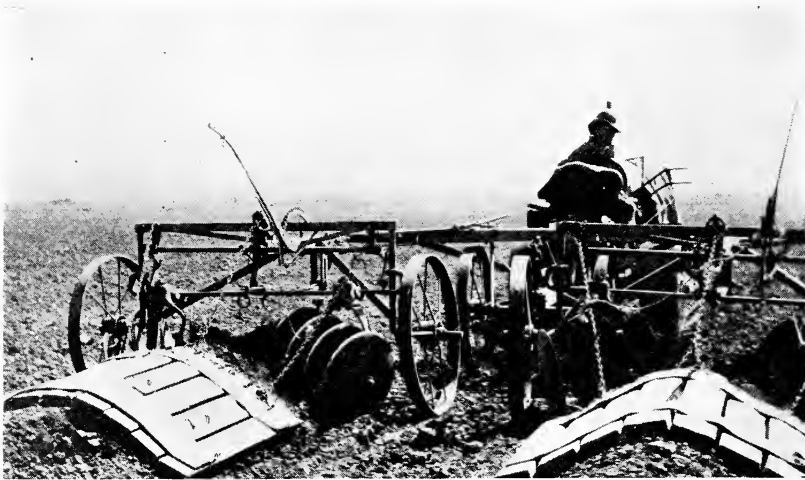
Fig. 10.—A board float attached behind the disks. (From Bul. 446.)
