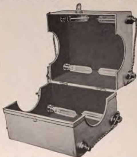
FIG. 60.—AUTHOR'S ELECTRIC LIGHT CABINET FOR JOINTS.
