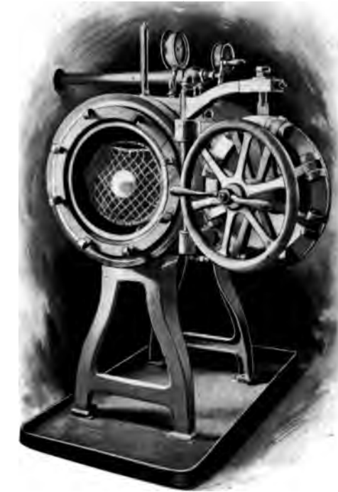
FIG. 22.—“The sterilizer devised by Col. John Fehrenbatch.”—REED (page 61).
