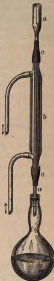
FIG. 9. — FLASK WITH REFLUX-CONDENSER.
