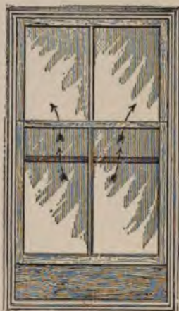
Fig. 2. Method of ventilating a room by raising the lower sash on a board. The arrows indicate the direction taken by the incoming air.
