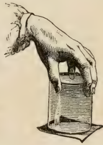
Fig. 12.—Atmospheric pressure under an inverted glass.
