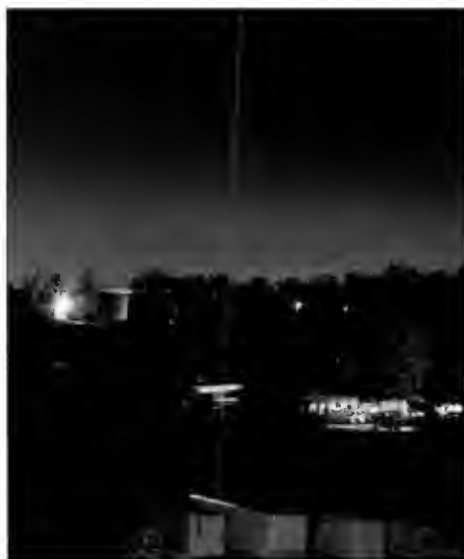
In this photo, the powerful laser beam from the STROZ-LITE lidar is pointed into the night sky above Goddard Space Flight Center. Laser light scattered back to the instrument from stratospheric molecules is analyzed to obtain ozone concentrations at various altitudes.
