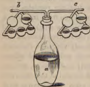
Schultze's experiment on SPONTANEOUS GENERATION.— a . Flask containing watery infusion. b . Potassa apparatus containing sulphuric acid. c . Potassa-apparatus containing caustic potassa.
