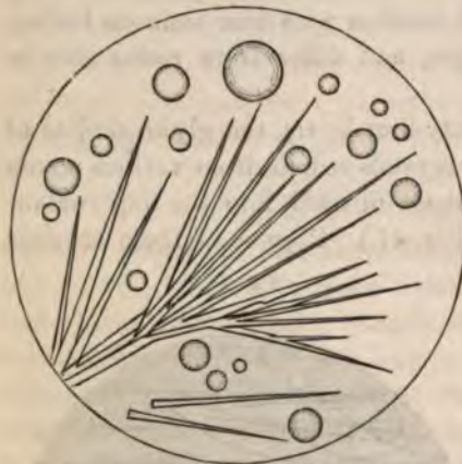
GLYKO-CHOLATE AND TAURO-CHOLATE OF SODA, FROM OX-BILE, after six days' crystallization. The glyko-cholate is crystallized; the tauro-cholate is in fluid drops.
