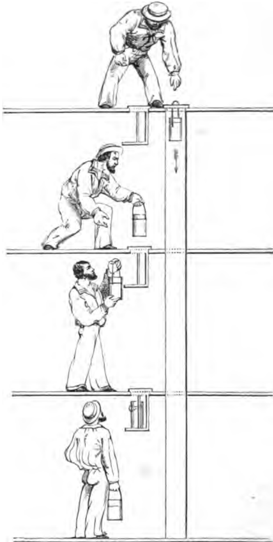
Illustration of the French mode of handing up Cartridges for the supply of the Batteries on the Decks of a first-rate Ship, and of returning the empty Cartridge Cases to the Orlop.
