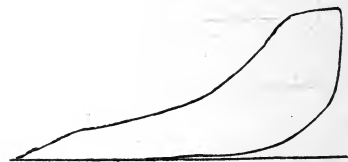
FIGS. 2,598 and 2,599.—Single valve cut off engine. For light and heavy loads, the initial steam pressure is about the same, and as the load increases, the point of cut off occurs later in the stroke. Compression becomes later as the cut off increases. The points of admission and release change also, but not so noticeably as the cut off and compression.
