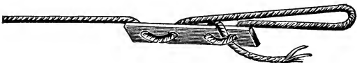
FIG. 2,542.—Connecting cord and method of attaching. The indicator should be connected to the engine cross head by as short a length of cord as possible. Cord having very little
