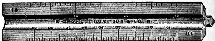
FIG. 2,519.—Triangular boxwood indicator scale. The six faces give six different scales corresponding to springs of like number.
