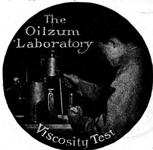
FIG. 2,165.— Fluidity or viscosity test. Viscosity represents the flowing quality of an oil and is determined by noting the number of seconds taken to pass a certain quantity of the oil at a specified temperature through a standard size orifice made for the purpose.
