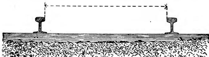
FIG. 1,891.— Gauge of track. This term means the distance between the inside edges of the heads of the rails, as indicated in the cut. The distance over the wheel flanges represent the gauge less the amount of play or clearance between the flange and rail. When deciding upon the gauge for a contemplated road, the following suggestions will be found helpful: If the line is to connect with any standard gauge road, the track should correspond and be of the standard broad gauge, which is four feet eight and one-half inches. If such connection be unlikely and narrow gauge is considered preferable, the standard narrow gauge should be adopted, which is three feet. The advantage of adopting one of these standard gauges is that, should it be desirable at any time to sell the equipment, a ready market can be found. For logging railroads the standard gauge of 4 ft. 8½ ins. is generally preferable, as the cars then can have long bolsters and can be heavily loaded without piling the logs too high. While some roads use the same gauge in curves as on tangents it is desirable in order to insure easy riding and reduce wear to widen the gauge in the curves. According to Trautwine, the gauge is usually widened by from 1/32 to 1/8 ins. for each degree of curvature, the maximum amount seldom exceeding one inch.
