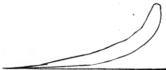
FIGS. 2,598 and 2,599.—Single valve cut off engine. For light and heavy loads, the initial steam pressure is about the same, and as the load increases, the point of cut off occurs later in the stroke. Compression becomes later as the cut off increases. The points of admission and release change also, but not so noticeably as the cut off and compression.
