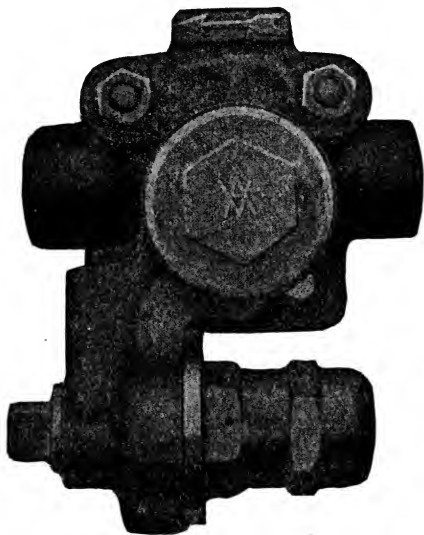
FIG. 2,014.—Westinghouse C-6 reducing valve. This valve is the well known feed valve that has been used for many years in connection with the G-6 brake valve, but in the ET equipment, it is attached to a pipe bracket. The only difference between it and the B-6 feed valve is in the adjustment, it being designed to reduce main reservoir pressure to a single fixed pressure, which in this equipment is, as already stated, 45 pounds. To adjust this valve , remove the cap nut on the end of the spring box; this will expose the adjusting nut, by which the adjustment is made. It is called a "reducing valve" when used with the independent brake and air signal systems, simply to distinguish it from the feed valve supplying the automatic brake valve.
