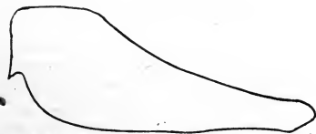
FIGS. 2,614 and 2,615.— Leaks indicated by compression line. The curvature of the compression line changes as the piston nears the end of the stroke; sometimes even forming a hook. This indicates the escape of steam from the compression space, either through the exhaust or past the piston.
