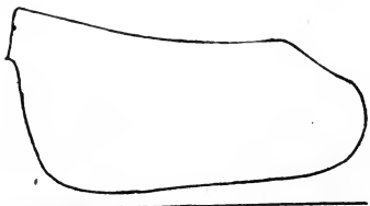
FIGS. 2,614 and 2,615.— Leaks indicated by compression line. The curvature of the compression line changes as the piston nears the end of the stroke; sometimes even forming a hook. This indicates the escape of steam from the compression space, either through the exhaust or past the piston.
