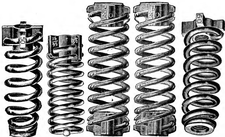
FIGS. 2,514 to 2,518.—Various indicator springs. Fig. 2,514, Richard Thompson; fig. 2,515, Schaffer and Budenberg; 2,516 and 2,517, Tabor, duplex; 2,518 Trill.
