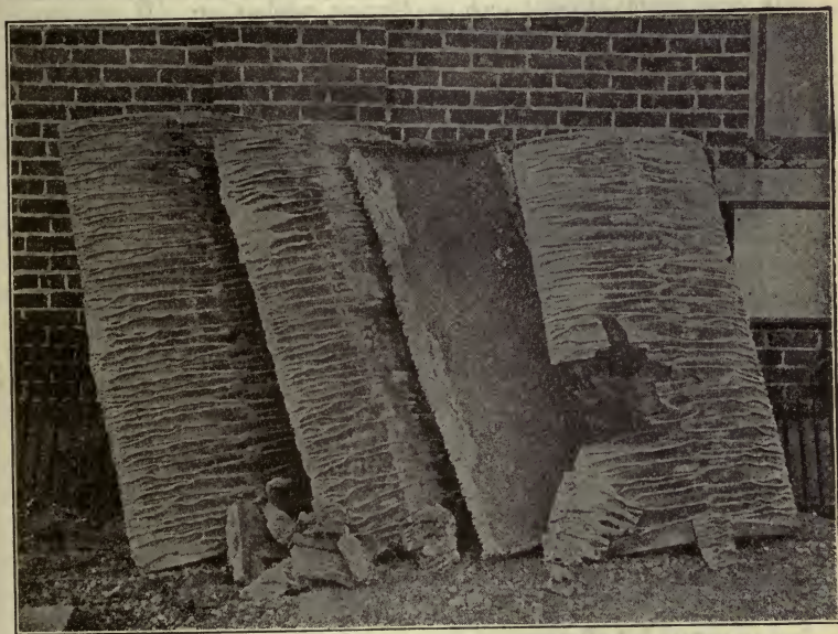
FIG. 4,119.—Pans for Hoppes exhaust steam feed water heater showing large amount of scale precipitated by heating the feed water and how the scale adheres to the underneath surface of the pans. The second pan from the right shows the deposit of scale on the inside or trough of the pan.
