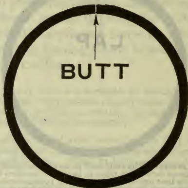
FIG. 4,947.— Butt weld process. Skelp used in making butt welded pipe comes from the rolling department of the steel mills with a specified length, width and gauge, according to the size pipe for which it is ordered. The edges are slightly beveled with the face of the skelp, so that the surface of the plate which is to become the inside of the pipe is not quite as wide as that which forms the outside; thus when the edges are brought together they meet squarely, as shown. The skelp for all butt welded pipe is heated uniformly to the welding temperature, in furnaces similar in general construction to those used in lap welding. The strips of steel when properly heated are seized by their ends with tongs and drawn from the furnaces through bell shaped dies, or rings. The inside of these dies is so shaped that the plate is gradually turned around into the shape of a tube, the edges being forced squarely together and welded. For some sizes, the pipes are drawn through two rings consecutively at one heat, one ring being just behind the other, the second one being of smaller diameter than the first. The pipes are then run through sizing and cross rolls similar to those used in the lap weld process, obtaining thereby the correct outside diameter and finish. The pull required to draw double extra strong (hydraulic) pipe by this process is so great, on account of the thickness of the skelp, that it is found necessary to weld a strong bar on the end of the skelp, thereby distributing the strain. With this bar the skelp is drawn through several dies of decreasing size, and is reheated between each draw until the seam is thoroughly welded. It is evident that the skelp is put to a severe test in this operation, and, unless the metal be sound and homogeneous, the ends will most always be pulled off.
