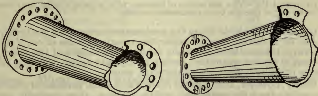
FIGS. 4,113 and 4,114.—Fractured Galloway tubes. In fig. 4,113 the upper flange is fractured all round the circumference and the lower, two-thirds around. At the prolongation of the fractures, cracks both superficial and otherwise were noticed. The appearance of the fractures seems to indicate that the metal was very brittle. In the tube, fig. 4,114, the upper flange is fractured at the beginning of the curvature for nearly the whole of the circumference.
