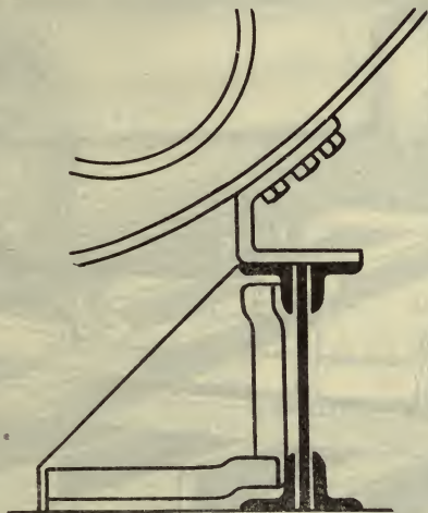
FIG. 4,456.—Horizontal marine boiler saddle. The weight of the boiler is supported on saddles or bearers which are attached to the structure of the ship. There are several of these saddles on each side of the boiler, each extending a little distance longitudinally to give a firm bearing.
