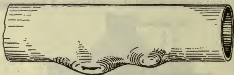
FIG. 4,108.—Tube from the lower row of a tubular boiler in a sugar refinery. On account of sugar in the boiler, the tube became overheated and gave away in the furnace. No elongation was observed at the place of the fracture.
