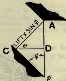
FIGS. 4,727 to 4,729.—Beveled valve and seat with diagrams, illustrating method of calculating valve opening area as explained in the accompanying note.
