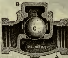
FIGS. 4,720 to 4,722.—Lukenheimer ball check valves. Fig. 4,720, anglé pattern; fig. 4,721, horizontal pattern; fig. 4,722, vertical pattern. This form of check consists of three parts, A , seat casting; C , ball; B , bonnet. It meets the requirements for users of this type of check valve, but is not desirable for sizes above 3 inches because of the high cost and weight of the ball.
