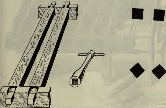
FIGS. 4,285 to 4,288.—Wrought iron grate bars and wrench. Fig. 4,285 plain bar made of iron of square section. These bars may be turned back and forth to shake the fire by means of the wrench, fig. 4,286, and may be placed in parallel positions, fig. 4,287, for large air spaces, or in oblique positions, fig. 4,288, for small air space. On page 2,409 is shown a built up bar composed of wrought iron plates spaced by thimbles or distance pieces and riveted or bolted as shown.
