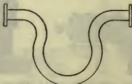
FIGS. 5,007 to 5,009.—Expansion bends. When the line is not too long and there is sufficient space this forms a good means of providing for expansion. The figures show several pipes arranged in parallel, although one large pipe may be and is frequently used, the single pipe requiring of course a larger radius of bend than the nest of small pipes.
