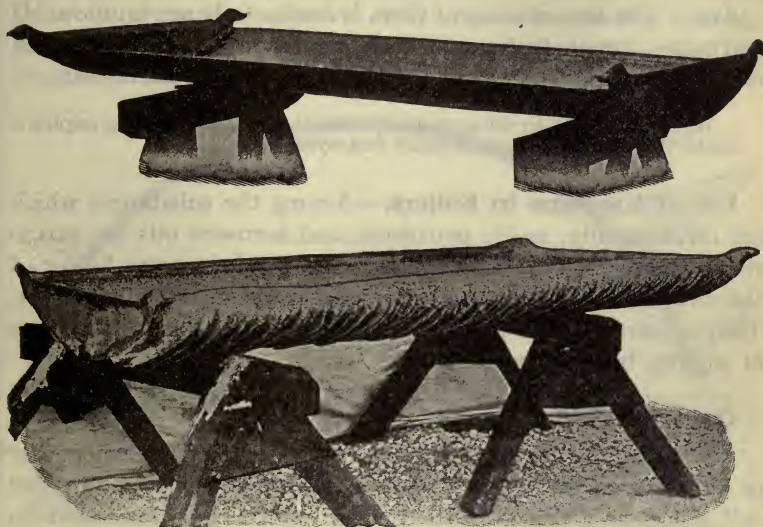
FIGS. 4,126 and 4,127.—Pans for Hoppe's live feed water purifier. Fig. 4,126, clean pan; fig. 4,127, same pan covered with scale after three weeks' use.
