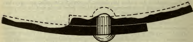
FIG. 4,109.—Corrosion of boiler shell along seam. This eating away of the plates is due to the chemical action of impure water. Gases absorbed by water, such as sulphuretted hydrogen and carbon dioxide are very active in the corrosion of boiler plates. Grease and organic matter also promotes corrosion.
