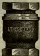
FIGS. 4,720 to 4,722.—Lukenheimer ball check valves. Fig. 4,720, anglé pattern; fig. 4,721, horizontal pattern; fig. 4,722, vertical pattern. This form of check consists of three parts, A , seat casting; C , ball; B , bonnet. It meets the requirements for users of this type of check valve, but is not desirable for sizes above 3 inches because of the high cost and weight of the ball.
