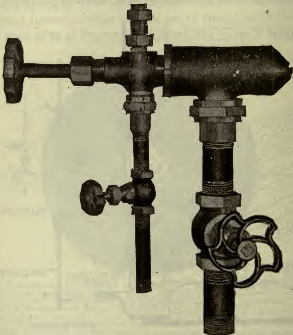
FIG. 4.381. Monarch all brass burner. It is a combination burner for either "high or low" pressure, and is adjusted by the center lock nut working backward or forward. The feed pipes are regulated with standard valves and the oil adjusted by needle valve.
