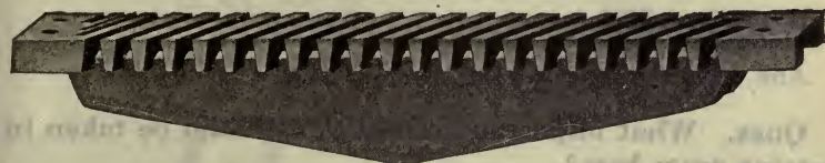
FIGS. 4,283 and 4,284.—Various grate bars. Fig. 4,283 Kelly herring bone or Tupper bar with recessed finger faces. These recesses become filled with ashes, which not only protect the surface from the intense heat of the incandescent coals but prevent slag from adhering to the metal. Fig. 4,284 Kelly bar with raised transverse fingers.
