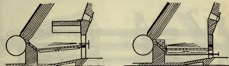
FIGS. 4,353 and 4,354.—Faulty and well designed furnace for Sterling boilers. In fig. 4,353 the flame is liable to impinge on the tubes.
