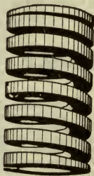
FIGS. 4,692 and 4,693.—American springs for brass and iron pop safety valves. Fig. 4,692, round type for brass valves 2 inches and under; fig. 4,693, rectangular type for brass and iron valves 2½ inches and over.
