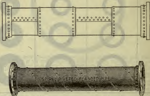
FIGS. 4,957 and 4,958.—Straight and spiral riveted steel pipe
