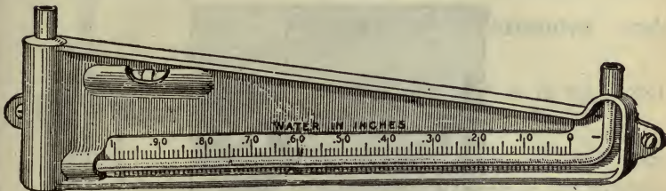
FIG. 4,833.—Inclined tube differential draught gauge. The fluid used is a special non-drying, non-evaporating, oil of known specific gravity. The incline and diameter of the tube are so proportioned that the draught may be read direct to one hundredth of an inch in term of distilled water. The indications are taken on one leg of the instrument only, and the movement of the fluid is ten to one.
