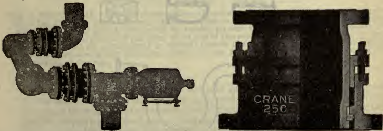
FIGS. 5,004 and 5,005.—Crane extra heavy swivel expansion joint for steam pressures up to 250 lbs. Fig. 5,004, method of placing swivel joints in a steam line; fig. 5,005, detail of joint. In construction , the male part of the joint is provided with a collar which bears against an internal ring cast on the sleeve and which prevents the two ends being forced apart by the steam pressure.
