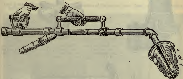
FIG. 4,843.—Goodfellow tube blower. The adjustable head fits and holds itself in different sizes of boiler tubes. Its adjustable steam nozzle delivers steam in lines oblique to the line of travel, drawing in hot air between the flanges, creating a whirling of steam air and grit, through and out of the tube. The adjustable handle enables the highest boiler tube to be reached from the floor, being so arranged that the steam hose may be attached at the middle or end of the handle.
