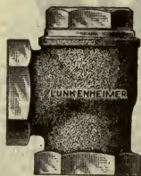
FIGS. 4,720 to 4,722.—Lukenheimer ball check valves. Fig. 4,720, anglé pattern; fig. 4,721, horizontal pattern; fig. 4,722, vertical pattern. This form of check consists of three parts, A , seat casting; C , ball; B , bonnet. It meets the requirements for users of this type of check valve, but is not desirable for sizes above 3 inches because of the high cost and weight of the ball.
