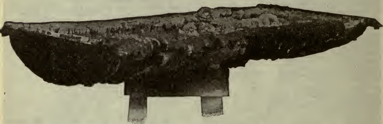
FIG. 4,120.—Another pan for Hoppes exhaust steam feed water heater showing large amount of scale precipitated both inside and outside of the pan.
