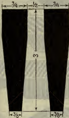
fig. 4,276.—Section through two finger straight bar, showing proportions. The bars should not be more than three feet long and should be thinner at the bottom than at the top. To maintain constant air spaces even after the top surfaces have worn down, the fingers are made the same thickness for about 1 inch from the top, being tapered from that point to the bottom of the bars, one about 3 inches deep in the middle, depending on the length and width, and have distance pieces at the center as at the ends to prevent twisting. The illustration shows \frac{1}{2} -inch air spaces. The size of the spaces and width of bar will depend on the kind of fuel used, varying for coal for \frac{1}{4} to 1 inch, depending on the size of the lumps.
