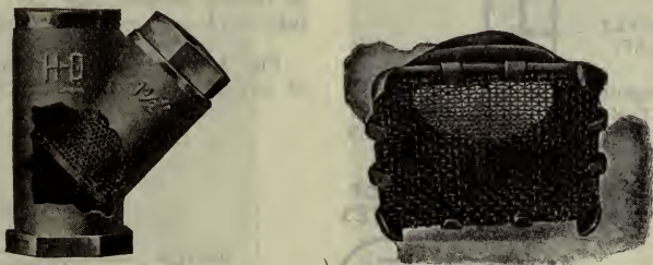
FIGS. 4,855 and 4,856.—Hayden & Derby strainers, for injectors or ejectors. Fig. 4,855, union strainer, this form screws on to the injector or ejector, and by removing the cap and screen can be withdrawn for cleaning. Fig. 4,856, flat strainer, a type suitable for vertical connections, as for instance, where an injector receives its water supply for a barrel or other vessel. Note the short legs at the corners which insure clearance between the strainer and surface on which it rests.
