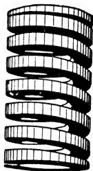
FIGS. 4,692 and 4,693.—American springs for brass and iron pop safety valves. Fig. 4,692, round type for brass valves 2 inches and under; fig. 4,693, rectangular type for brass and iron valves 2½ inches and over.
