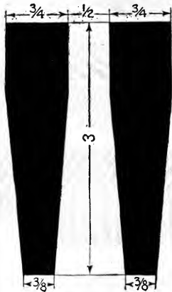
fig. 4,276.—Section through two finger straight bar, showing proportions. The bars should not be more than three feet long and should be thinner at the bottom than at the top. To maintain constant air spaces even after the top surfaces have worn down, the fingers are made the same thickness for about 1 inch from the top, being tapered from that point to the bottom of the bars, one about 3 inches deep in the middle, depending on the length and width, and have distance pieces at the center as at the ends to prevent twisting. The illustration shows \frac{1}{2} -inch air spaces. The size of the spaces and width of bar will depend on the kind of fuel used, varying for coal for \frac{1}{4} to 1 inch, depending on the size of the lumps.
