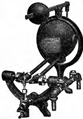
FIG. 4,937.—Bundy return trap. In operation when the bowl fills, it tilts and opens the valve admitting steam at boiler pressure, thus equalizing pressure in trap and boiler, and since the trap is placed above the water line, the water will pass by gravity from the trap into the boiler. To re-adjust. Place the counterbalance ball at a point on the lever where it will easily raise the empty bowl. See that the lower lock nuts which are touched by the sleeve are set just high enough on the valve stem to effectually close the steam valve without injuring disc or seat. Also that the upper set of locknuts are adjusted so that the bowl will have some headway on its downward stroke before engaging the ring to open the valve. Some lost motion must be maintained between the two sets of lock nuts, so the bowl may gain headway either up or down before the sleeve touches the lock nuts, thus opening and closing the valve with a quick movement.
