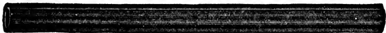
FIG. 4,748.—Scotch water gauge glass. Usually carried in stock in sizes from \frac{1}{2} to \frac{3}{4} ins. diameter and from 10 to 24 ins. in length.
