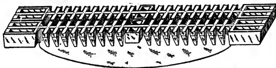
FIG. 4,269.—Fish bone type of grate bar. The illustration shows two of these bars side by side.
