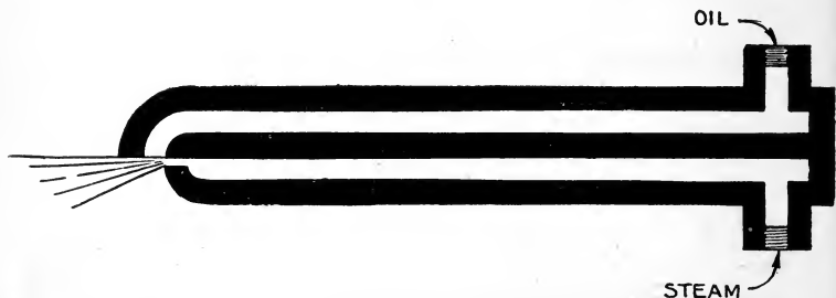
FIG. 4,358. Atomizer burner. The oil is brought through an orifice directly across the path of the jet of air or steam and is "brushed" off by the latter and sprayed.
