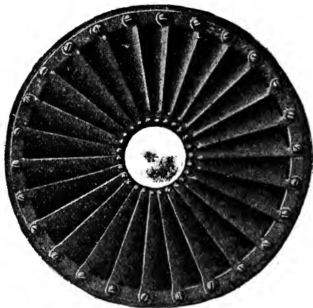
FIG. 4,379. Peabody and Irish impeller or air register. In a paper read before the Society of Naval Architects and Marine Engineers, Mr. Peabody says: "Great delicacy is required in introducing the air for combustion, very slight changes affecting the results in unsuspected ways, and while almost any method may result in smokeless combustion, maximum economy and capacity can be secured only by careful and intelligent design. It is not necessary to give the air a whirling motion but, judging from our rather exhaustive experiments, better gas analyses are secured, lower air pressures are required, and less refinement of adjustment is needed if the air be brought into contact with the oil spray with the right sort of a twist. We have found the impeller plate, illustrated on this page, most effective in accomplishing this mixture, and our most satisfactory results have been obtained with it."
