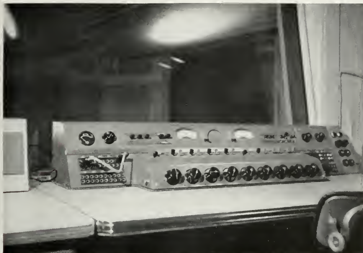
Western Electric, 6-mike mixing console in control room for main sound studio at Fulton Recording Company. Auxiliary panel at right-hand end of console contains special push-button controls for operation of the Ampex tape recorders.
