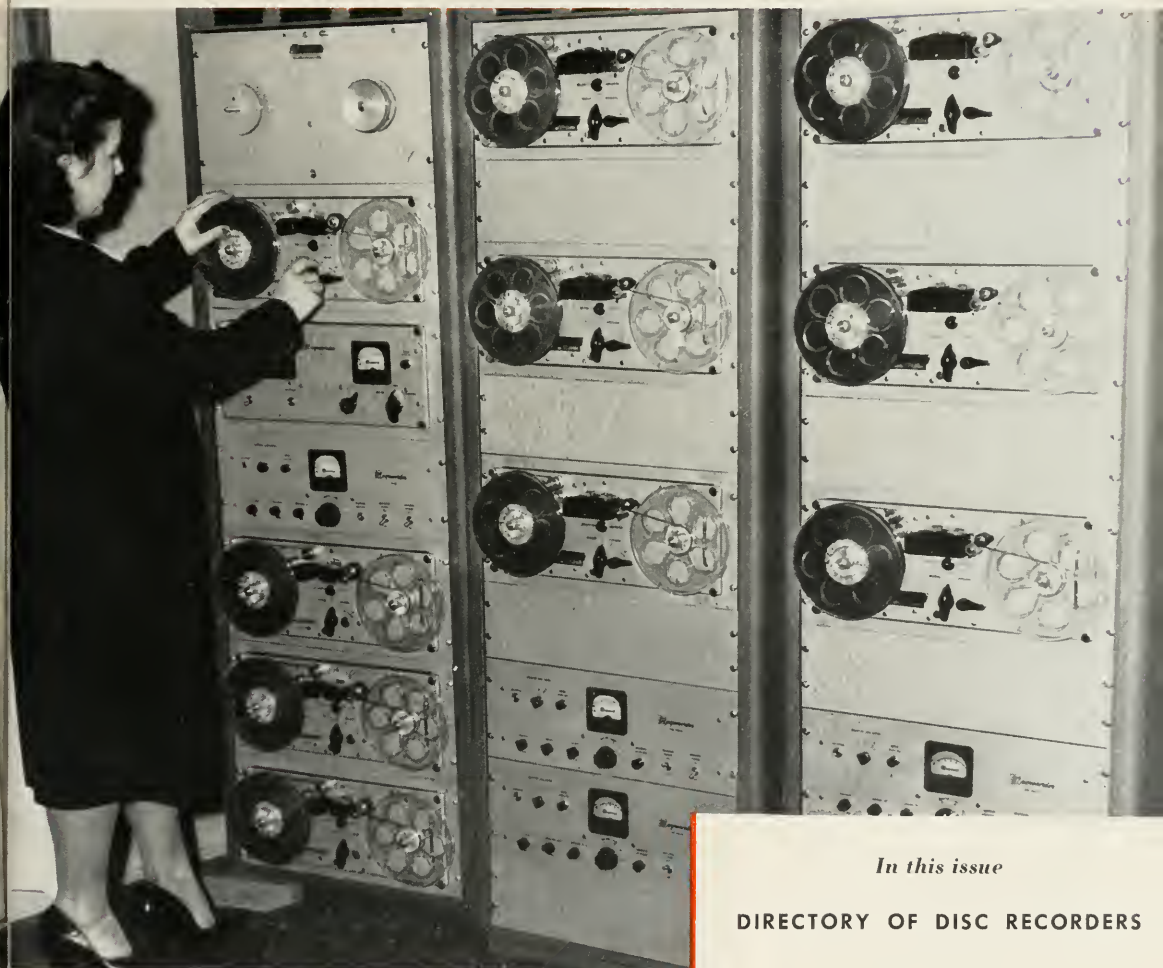
Ten rack-mounted Magnecord tape recorders arranged for full range duplication of pre-recorded "Magnerecordings by Vox", now being offered commercially by MaVoTape, Inc. All recordings are made on plastic base Audiotape. Story on Page 3.
