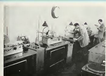
An engineer at Universal Recorders checks the depth of cut, the condition of the stylus and the distance between each groove through a microscope.
