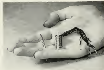
Close-up view of 5 unit recording head assembly for CRM-15 multiple-channel recorder. Three of these units are used to give full 15-channel capacity.
