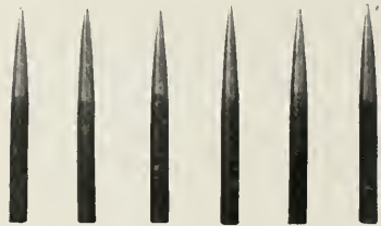
Fig. 1 — When steel playback points have been shadowgraphed, the complete uniformity of the styli is assured.
