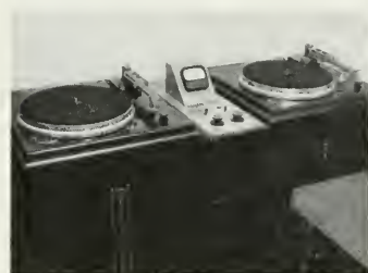
Fig. 2—Dubbing and playback tables, mounted on special rubber cups and cork sheeting to eliminate building vibration.
