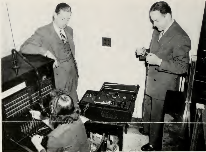
Edith Hingley, KDKA-Pittsburgh switchboard operator listens while T. C. Kenney, Chief Engineer, and J. E. Baudino, General Manager, explain the technical phases of the station's telephone answering gimmick. A magnetic tape recorder specially rigged to the outlet's switchboard played back recorded "hellos" of network stars to incoming callers—KDKA's way of hypoing listener interest in web shows.
