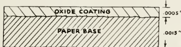
Fig. 2. Showing how microscopic surface irregularity of base can introduce coating thickness variations and hence modulation noise.
