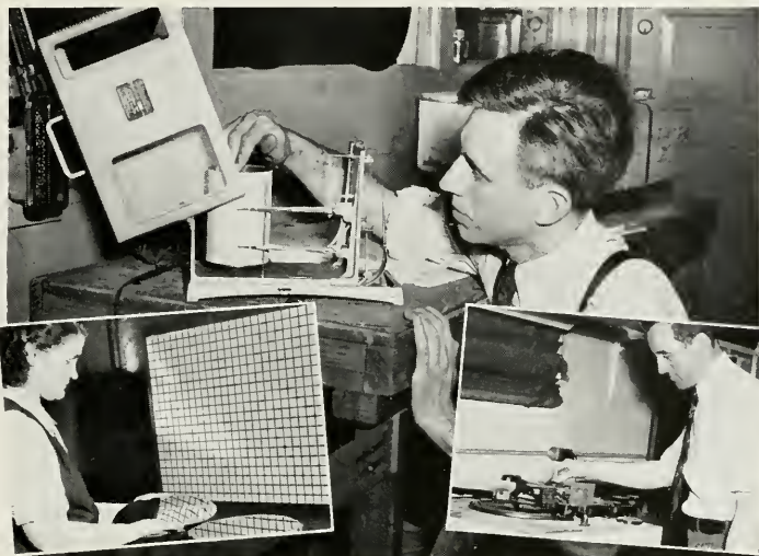
Scenes from Audio Devices' movie "Audiorecords—They Speak For Themselves." Above: Engineer examining hygro-thermograph. Left Inset: Inspector testing aluminum bases for flatness with mirrorgraph. Right Inset: Engineer operating machine which tests wearing qualities of discs.
