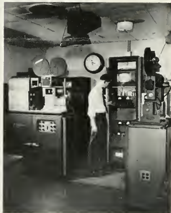
Fig. 3. One of ABC's kinescope recording rooms at Station WJZ-TV, New York, showing a matched pair of 16mm sound film recording units. Each unit consists of a Wall camera and special Maurer optical recorder mounted on an RCA Kinephoto recording monitor.
