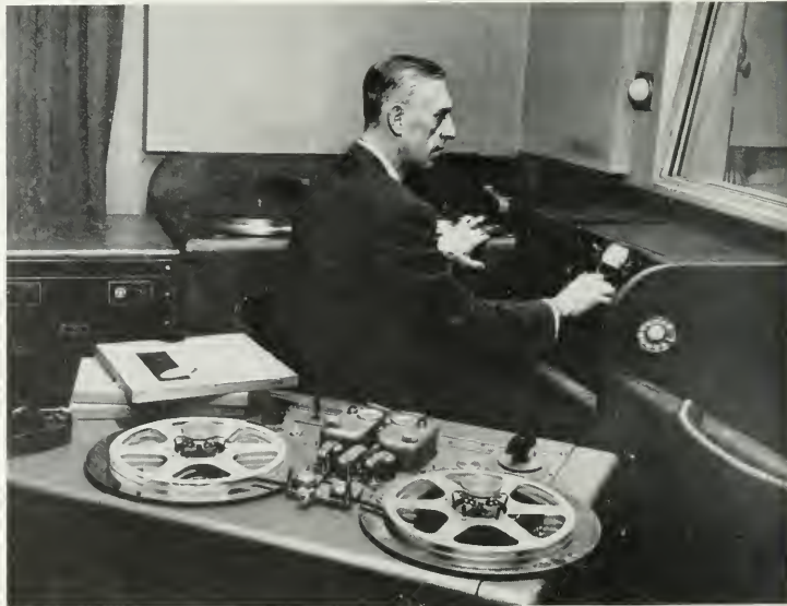
Ralph Schlegel, Recording Supervisor, at the control console in one of WOR's many sound-proof, air-conditioned recording rooms. A Rangertone tape recorder is shown in the foreground.
