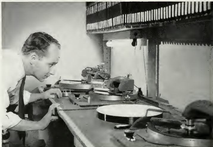
Dave Ficker keeps an eagle eye on the bank of four cutters, making acetate duplicates of a tape recording. Magnecorder tape recorder is shown on the cover illustration.
