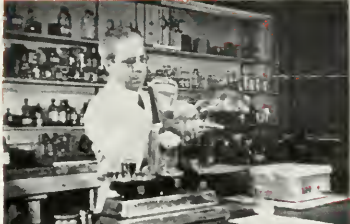
Laboratory demonstration showing precipitation of magnetic oxide used in Audiotape coating.
