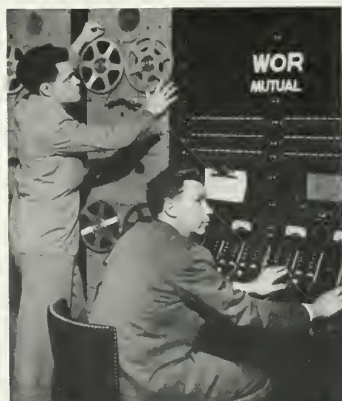
Another view of the WOR "Mutual Room" shown on this month's cover. This installation includes a bank of 12 rack-mounted Magnecorders, 6 on each side of the control console shown above.
