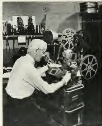
Fig. 5. Engineer Edward J. Green demonstrates operation of Movieta sound film editing equipment, in one of the WJZ-TV editing rooms. Film at left is used for sound track, and at right, for picture. Any parts to be removed are marked on both picture and sound track, to be cut and spliced later.
