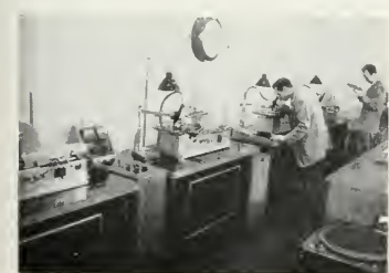
An engineer at Universal Recorders checks the depth of cut, the condition of the stylus and the distance between each groove through a microscope.
