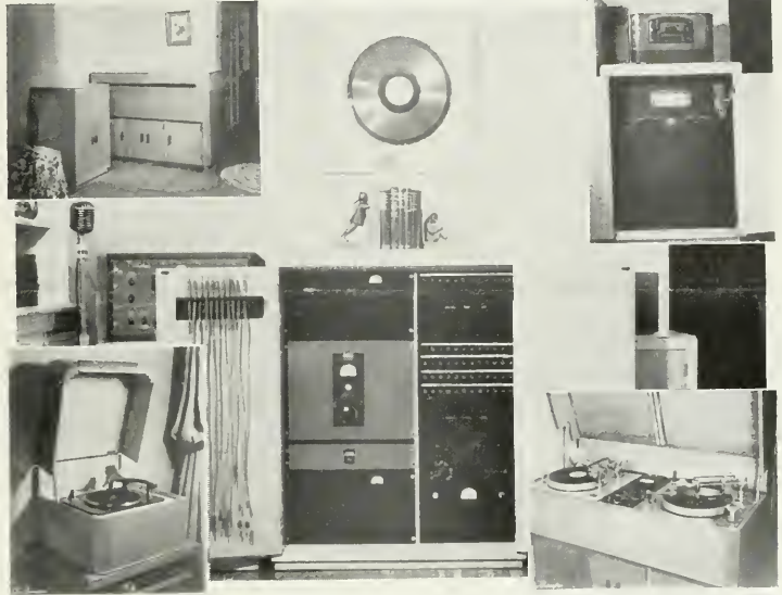
Occupying an attractive corner in Larry Ruddell's living room (Larry is ABC's disc chief) is this amplifier rack, which contains 6 channels of recording equipment and the master control board. Other units in the room, pictured clockwise: New Garrard RC-60 record changer atop a 16" record file cabinet; Match ply-wood cabinets housing test equipment and recording lathes; Incompleted power supply and tuner rack; Inside view of recording tables, which includes equalizers, transfer keys, VI meters, etc.
