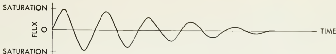
Figure 2. Hysteresis diagram showing how magnetic condition of head is carried in opposite directions, but with successively decreasing amplitude, finally ending at zero.
