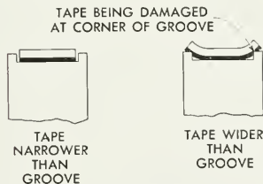
Fig. 4. Diagram of worn heads showing the effects of normal variation in tape width.
