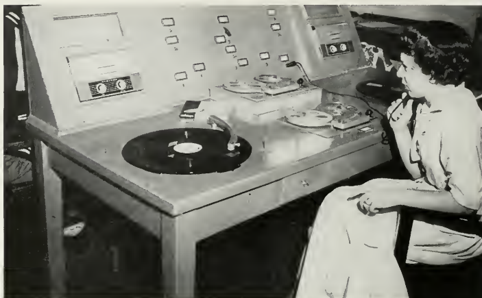
Control table in the "listening room" at Mt. San Antonio College. Built by Mr. Wesley L. Lewis, it includes two tape recorders and two disc recorders, with switching facilities for feeding either tape or disc programs to any or all student listening stations.
