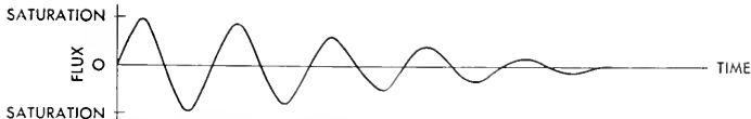
Figure 2. Hysteresis diagram showing how magnetic condition of head is carried in opposite directions, but with successively decreasing amplitude, finally ending at zero.
