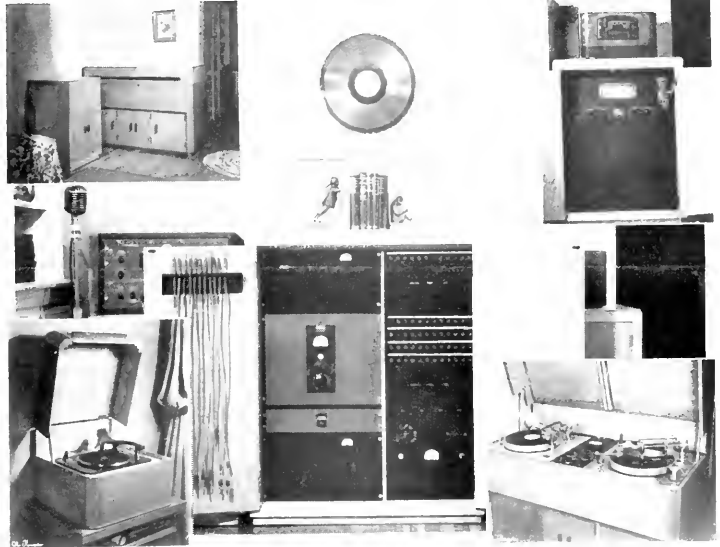
Occupying an attractive corner in Larry Ruddlell's living room (Larry is ABC's disc chief) is this amplifier rack, which contains 6 channels of recording equipment and the master control board. Other units in the room, pictured clockwise: New Garrard RC-60 record changer atop a 16" record file cabinet; Match ply-wood cabinets housing test equipment and recording lathes; Incompleted power supply and tuner rack; Inside view of recording tables, which includes equalizers, transfer keys, VI meters, etc.
