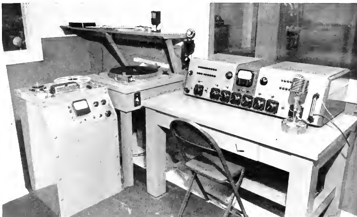
Part of the control room at Kay Bank Recordings, showing RCA 76B2 console with talk-back mike to studio, Ampex recorder for studio tape work, and transcription turntable.
