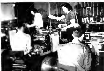
Part of the slitting room, where the large coated rolls are slit to the required width and wound on reels or hubs.
