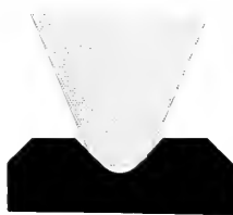
Fig. 1 Stylus-Groove Relation for Proper Tracking
