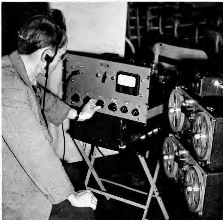
Typical recording setup as used for making rehearsal tests during class session of the Berkeley Opera Workshop. Equipment shown includes two portable Magnecorders and separate amplifier chassis.
