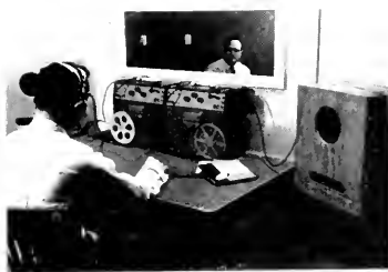
Stereophonic recording equipment in use at Psychology of Music Laboratory, University of Kansas. Set-up shown includes two Pentron recorders in tandem, matched right and left field speakers, and binaural headset.
