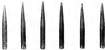
Fig. 2 — Typical points rejected in shadowgraphing. The first two points are hooked, the second two are broken off at the tip and the third two have split points.
