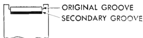
Fig. 5. Diagram showing two consecutive stages of head wear resulting from the use of successively narrower tape widths.
