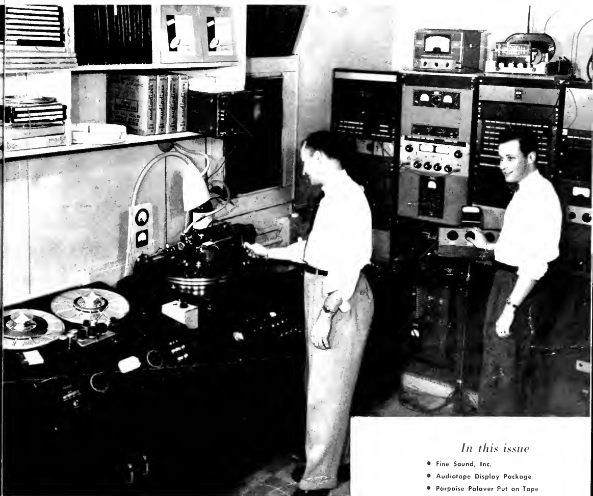
Fine sound in the making, by Fine Sound, Inc. George Piro (left) tends the Margin Control while cutting a long playing master, as Bob Fine (right) adjusts the recording level. Equipment shown includes a Fairchild tape recorder and Fairchild Model 523 Disc Recorder with Miller cutterhead specially made to Fine Sound specifications. Story on Page 2.
