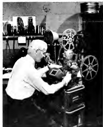
Fig. 5. Engineer Edward J. Greene demonstrates operation of Movieta sound film editing equipment, in one of the WJZ-TV editing rooms. Film at left is used for sound track, and at right, for picture. Any parts to be removed are marked on both picture and sound track, to be cut and spliced later.
