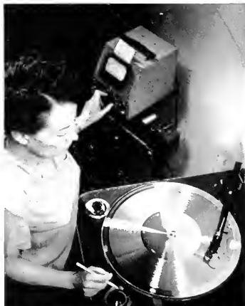
Complete audio testing of all metal "mothers" is just one of Allied's many exacting quality-control measures. In addition, every tenth pressing is played all the way through, to catch any imperfections which might possibly develop in the matrix or stamper.
