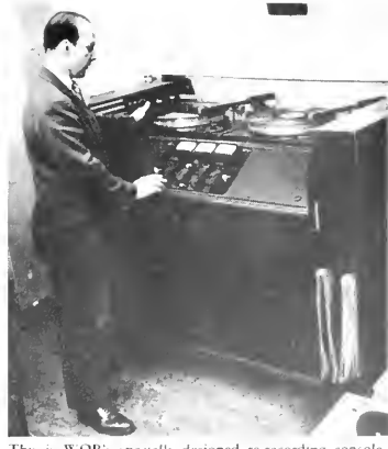
This is WOR's specially designed re-recording console, with which it is possible to make disc "copies" which are actually superior in quality to the original.
