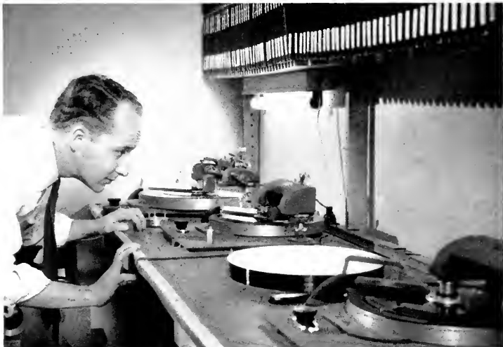
Dave Ficker keeps an eagle eye on the bank of four cutters, making acetate duplicates of a tape recording. Magneorder tape recorder is shown on the cover illustration.
