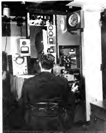
Fig. 7. This kinescope camera—one of a bank of similar machines at NBC—records the picture separately on 16mm photographic film. Duplicate films are made of every recorded show.
