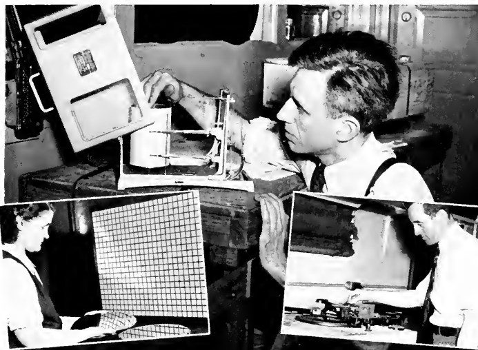
Scenes from Audio Devices' movie "Audiodiscs—They Speak For Themselves." Above: Engineer examining hygro-thermograph. Left Inset: Inspector testing aluminum bases for flatness with mirrorgraph. Right Inset: Engineer operating machine which tests wearing qualities of discs.
