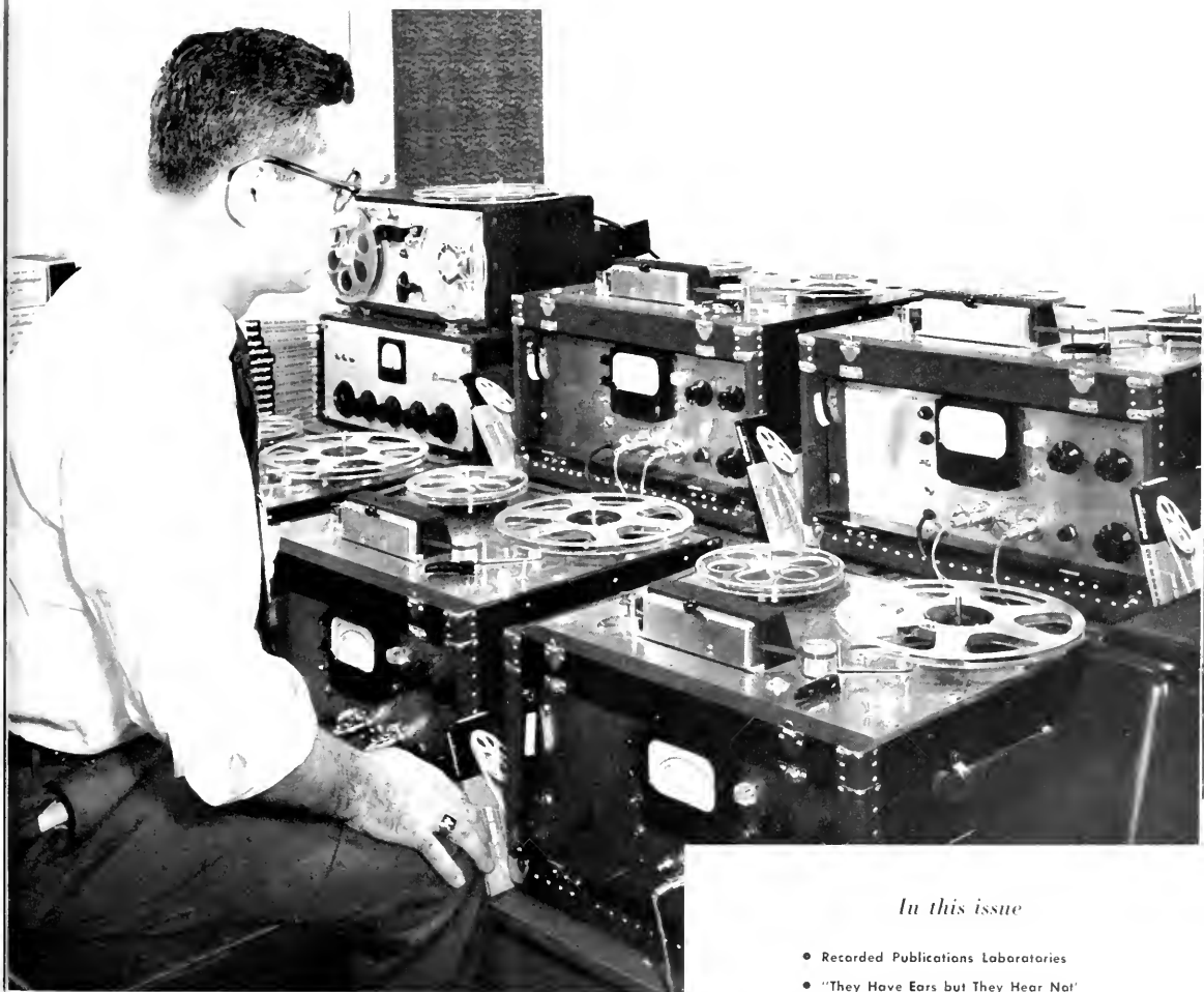
Multiple recorder set-up for duplication of recorded tapes at Recorded Publications Laboratories, Camden, N. J. Story on Page 2.
