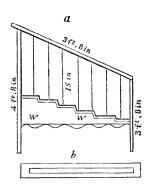
measurement, is 4 ft. 8 in. at the back; 3 ft. 8 in. in front; 3 ft. 8 in. in depth, from front to back; and 15 in. from the shelves to the glass top light: the rise between the shelves is two inches, and the whole
