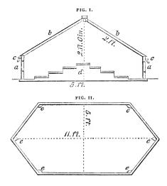
Fig. 1. a a, ventilators, of which there are eight; b b, sashes, with hinges at top; c c, handles, two on each side; d, stage, for holding 130 pots.
