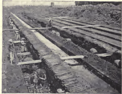
FIG. 221.—Method of Removing the Cement Copper.
