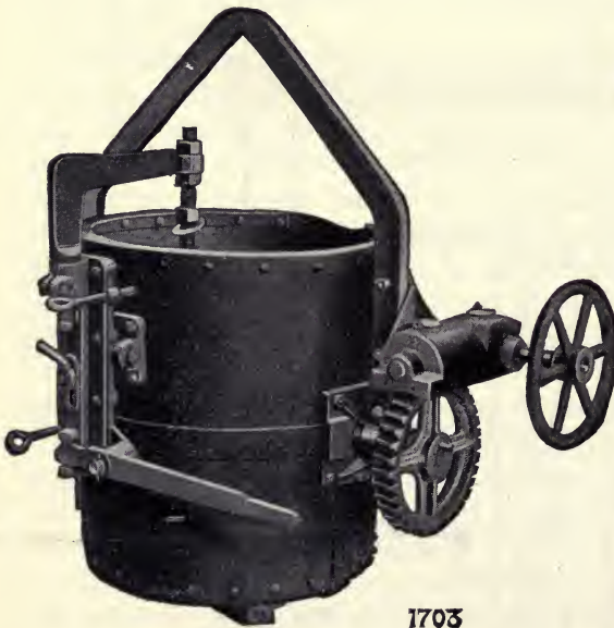
FIG. 171.—Worm-gear Bottom-tap Ladle, Pittsburg Elect. Furnace Corp.
