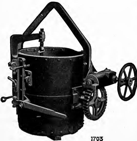
FIG. 171.—Worm-gear Bottom-tap Ladle, Pittsburg Elect. Furnace Corp.
