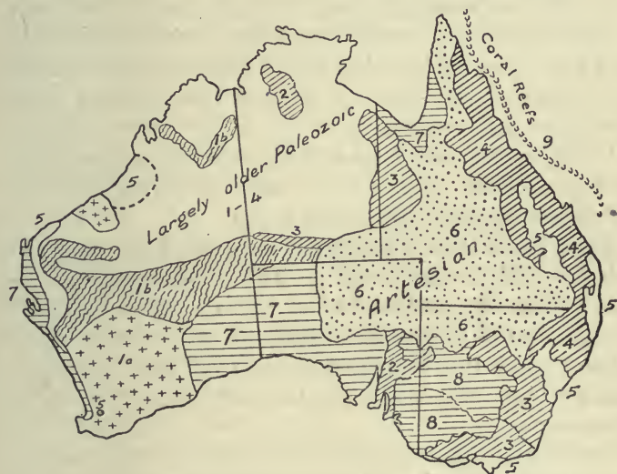
FIG. 5. Geological Sketch-map of Australia. 1 = Gneisses and Granites (Archean); 2 = Cambrian Sediments; 3 = Silurian Slates, &c.; 4 = Devonian and Carboniferous; 5 = Coal-measures (Permian, &c.); 6 = Cretaceous Artesian Basin; 7, 8 = Tertiary; 9 = Pleistocene Coral Limestone. (All generalized.)
