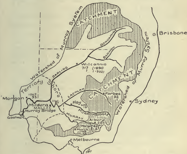
FIG. 42. The Murray-Darling Basin (after R. McKay) showing the effective Catchment Area (shaded). The greatest and least annual flow (in thousand million gallons) at the important river towns is indicated also.
