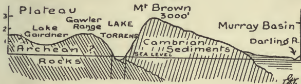
FIG. 25. Section across the Cambrian Divide, about the latitude of Lake Torrens, showing the Rift Valley occupied by the latter Lake.
