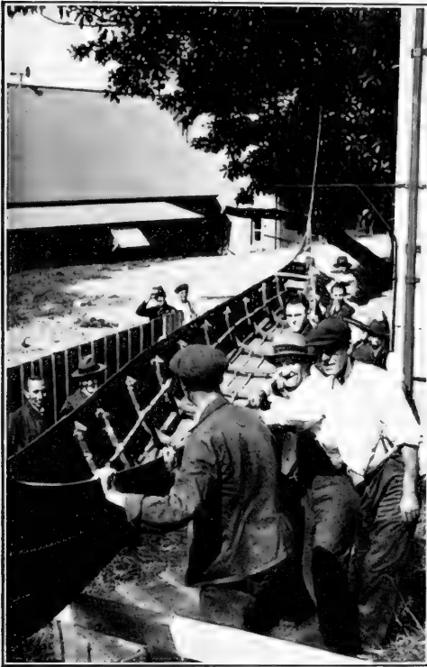
The canoe in process of transference. Note its beautiful lines and sound construction. Seats rest upon the bearers attached to the ribs.
