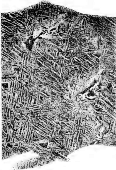
A portion of the etched surface of the "Delegate" meteorite (siderite) showing Widmanstätten figures. This is reproduced direct from a contact print taken from the meteorite.
