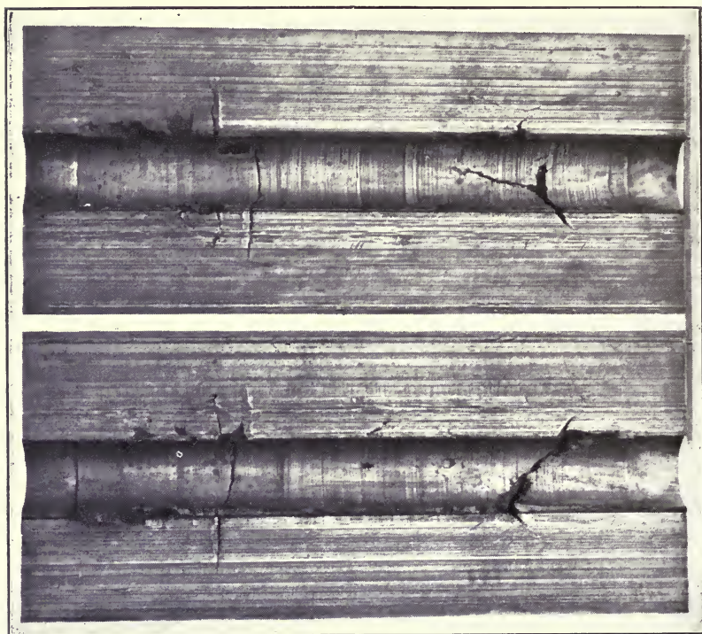
FIG. 8. — SECTION OF STEEL SHAFT SHOWING IMPERFECTIONS IN FORGING.
