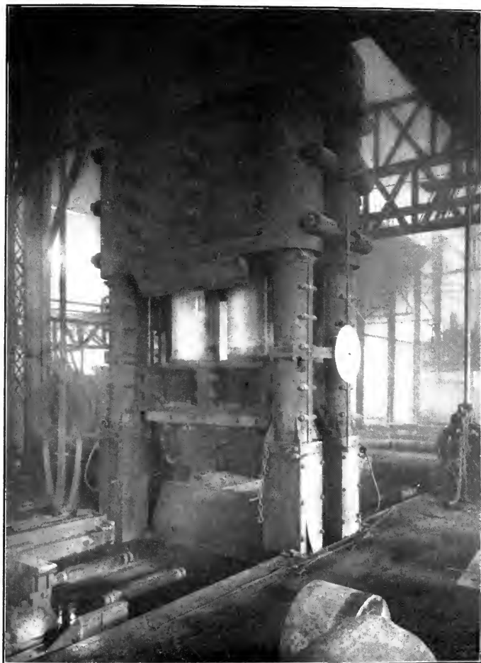
FIG. 10. — FOURTEEN THOUSAND TON HYDRAULIC FORGING PRESS, BUILT BY THE BETHLEHEM IRON COMPANY. TWO CYLINDERS, EACH FIFTY INCHES IN DIAMETER.
