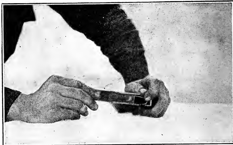
With the left hand hold the magazine spring in position. Slide the magazine base fully home.
