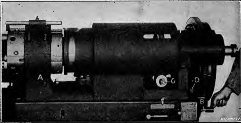
Fig. 9. Turret-slide of Cleveland Automatic, which is Adjusted Along the Bed to Suit the Various Lengths of Work and Turret Tools
