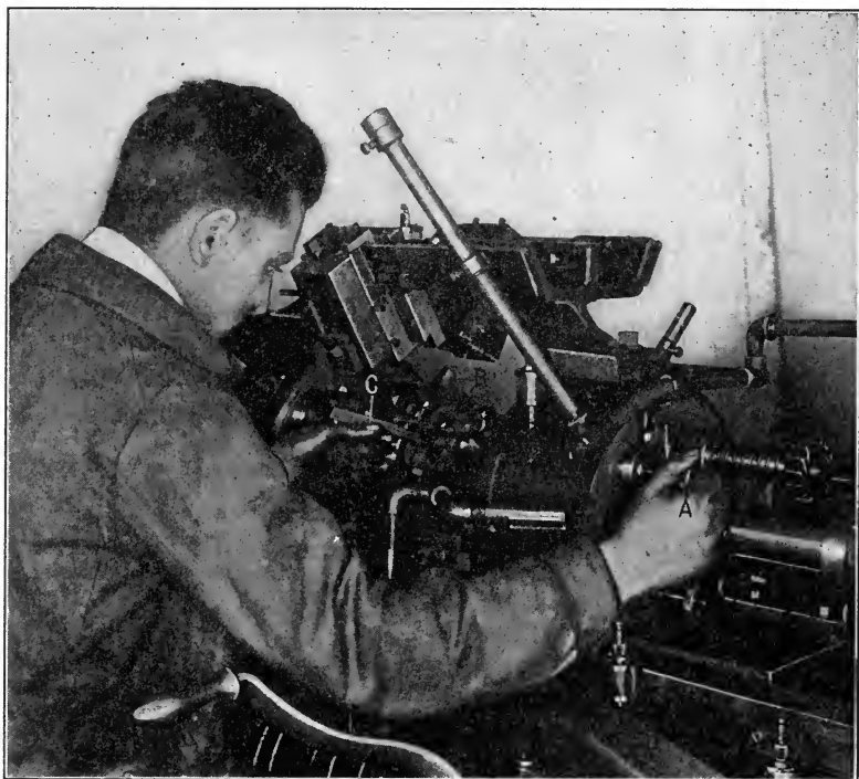
Fig. 18. Setting the "First" Position Box-tool to turn to the Required Distance on the Work
