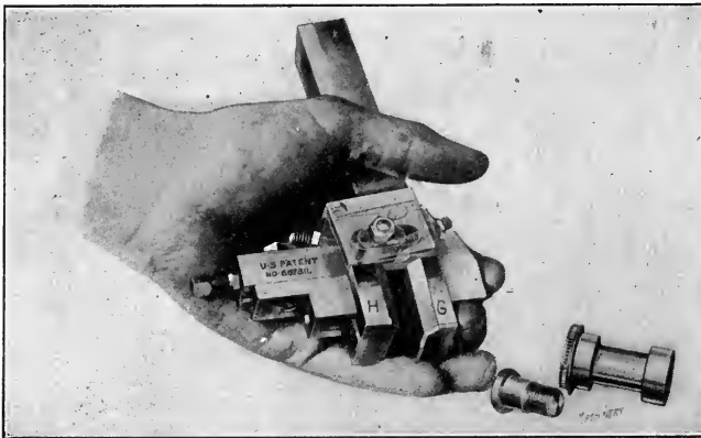
Fig. 33. Shaving Tool used on the "Acme" Multiple-spindle Automatic Screw Machine, and Examples of Work
