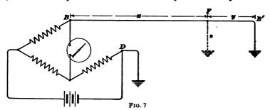
the resistance z of the fault remaining the same during both measurements. The farther the fault lies from the tested station, the more accurate will be the result; so the more reliable result will be that obtained by making the test from the end farthest from the fault. However, if two faults exist, the best result is obtained by making the test at the end
