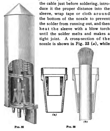
Fig. 33 (b) shows a completed joint. A skilled plumber is not necessary to make this joint; it is therefore especially useful for small companies that do not have enough steady work for a regular cable splicer. The lower part c of the combined cable box and terminal shown in Fig. 32 is made separate for use as a junction box only; the upper part
