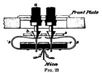
As the sliding plate moves down and all the holes in it come just opposite the shoulders on all the pushbutton rods, all the pushbuttons that may have been pressed in are pushed out by their springs 2,5, Fig. 23, to their normal positions as the hook
