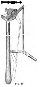
and that its leverage exceeds that of any other trimmer. It is stamped from sheet steel, is almost unbreakable, and will stand very rough treatment.
