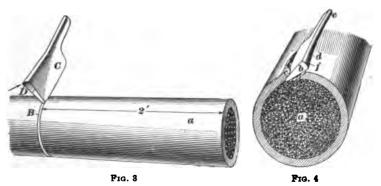
arrow, so as to give it a tangential motion. In this way, the sheath is cut without the knife being allowed to cut into the conductors. This groove having been cut, a longitudinal incision is made from it to the cable end. The method of holding the knife for this work is shown in Fig. 4. As
