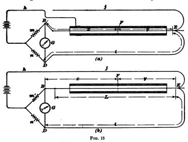
is not available, but where two good wires of any size and material, either inside or outside the cable, are available, the following modification, made by H. W. Fisher of the Murray loop test, may be used. It must be possible to connect 165—15
