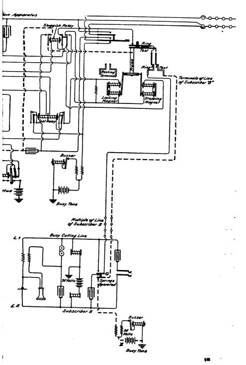
though the desired subscriber were on another line. The selector brushes J, Fig. 14, are caused to advance to a pair of revertive terminals bearing the number of the calling line, of which only the ringing terminal is connected to the ringing side of its own line. The ring selector brush is brought into contact with the said revertive line terminal, which is permanently connected with the L1 side of the circuit, instead of being carried through the rotary movement springs S of the selector.
