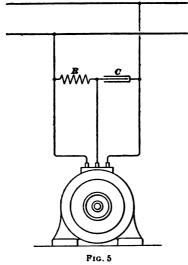
22. Speed Regulation of Induction Motors.-The induction motor tends to run nearly in synchronism with the alternator that supplies it with current. Its speed can never quite reach synchronism, because it always takes some power to make up for the friction losses, etc., even if the motor is unloaded. is also evident that the speed cannot rise above that of synchronism, and that with the exception of the slight
