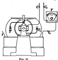
show a deflection. If the ground were complete, that is, a *dead ground*, the deflection would show the full voltage of the circuit  $CC_1$ .
