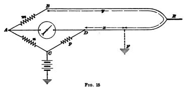
known. The loop BED is connected to the bridge, as shown in Fig. 15, and a balance obtained. Then,
