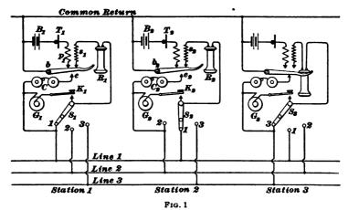
of numbers. The system of electrical connections is in no wise affected by this, the button being merely shifted from the position it would ordinarily occupy to the first position because it is more convenient to have it there. The commonreturn wire runs through all of the stations with the other line wires.
