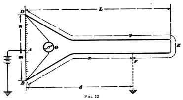
locating a ground on a line wire consists in using a slide wire in place of the two adjustable arms of a Wheatstone bridge in the Murray loop method. In Fig. 12, BD represents a wire of uniform resistance stretched over a
