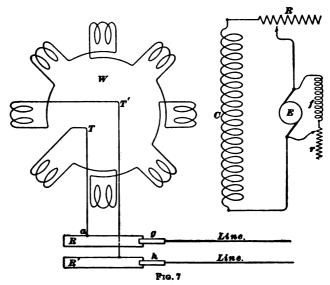
associated with it for exciting its field. In Fig. 7 is shown a diagram of connections of a simple alternating-current dynamo with a much smaller direct-current machine for exciting the alternator fields. W represents the armature winding of the alternator, the terminals T, T' of which are
