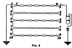
lated and open, and tests for the grounded wire. When found, he knows it to be conductor 1 and the wire twisted with it he knows to be conductor 2. Then, connecting one terminal of his testing set to wire 2
