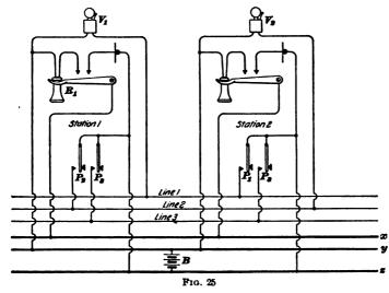
would be due merely to cross-talk as it were, caused by the internal resistance of the common battery B to which both talking circuits are connected in parallel.
