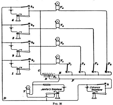
the common-return wire C, and battery. It will usually be necessary in order to place a telephone in each apartment to run a third wire D or to use a ground return in its place. In each apartment, there is a simple telephone with a transmitter and receiver in series, a push button and a battery
