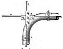
Where it is desirable to turn a cable around a corner where there is no pole, the arrangement indicated in Fig. 41 may be used. The cable is bent to the smallest possible radius and cable clips d, e are attached as near the bend are two three-bolt clamps e at
