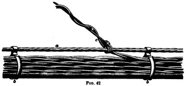
are run through the rings at any time by a man who rides in a carriage, which is a seat suspended on rollers from the messenger wire. It is also quite common to use a single steel wire of sufficient size in place of the stranded messenger wire shown. With this system, it is claimed that long spans, short poles, and smaller-sized service wires, which are subject to less mechanical stresses, may be used.
