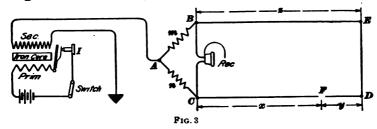
ends E, D are joined together in any convenient manner. A telephone receiver is connected across the points B C.
