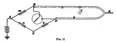
and bad wires joined together. Then connect the loop so formed to the bridge, as shown, in Fig. 9, for the Varley loop test, and measure the resistance of the loop. Let this resistance be R. Evidently, R = x + y. Then connect the loop and battery as in Fig. 11, thus having really only two adjustable arms, because A C and CD form only one arm now. F is now the junction between the arms x and y. When the bridge is balanced, we have
