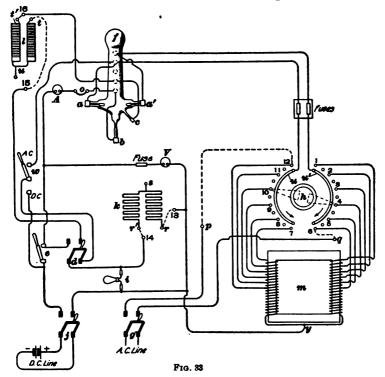
load, whatever it may be, will occupy the position now held by the storage battery. The rectifier is started in the same way as before, but in this case the starting current is alternating and flows through g-w'-d'-l-c-b-d-i and k in parallel-y-m-g', Fig. 32 (a).
