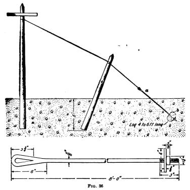
rock, a hole is blasted. This takes a great deal of time and is very dangerous and expensive. It is impossible to blast a hole of small diameter. When a sufficient depth is reached, the hole is funnel shaped, being possibly 3 or 4 feet in diameter at the top and tapering to an approximate point at the bottom. With the method illustrated, all that is necessary is to drill five  $1\frac{1}{4}$ -inch or  $1\frac{1}{2}$ -inch holes in the rock as
