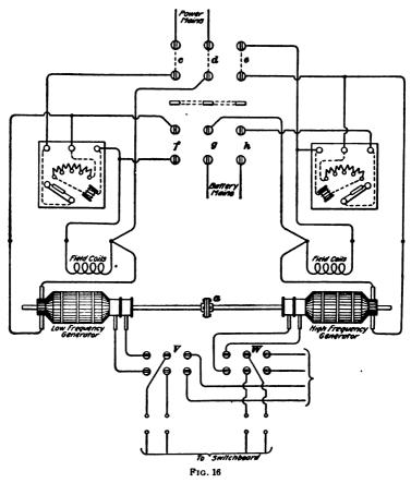
armatures and field coils of two dynamotors, whose shafts are mechanically coupled together at a, are connected with automatic-release starting rheostats and a three-blade double-throw switch, in such a manner that the left-hand machine, when supplied with current from the power mains, will run
