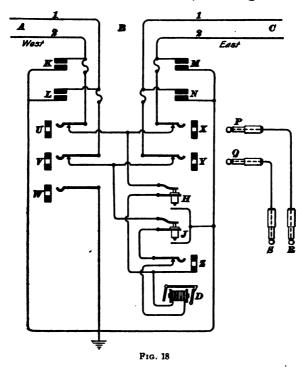
the operator is directed to open west, which is done by withdrawing plugs P, Q from jacks X, Y, and inserting them in jacks U, V. If no noise can now be heard at A, the trouble is evidently in office B, probably in the carbon arresters or heat coils. If no noise can be heard when the line is open east, only the operator is instructed to *strap through*, that is, insert plug P in jack X, R in U, Q in Y, and S in V, which cuts out the heat coils H, J and the drop D. This process is
