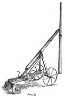
sort of a power appliance, such as a gasoline engine or electric motor, is placed on the front to raise the pole, instead of the winch, which is shown in this figure. The clamp that is used to hold the pole will grip the pole automatically, and loosen itself when the pole is set in the hole. When it is required to take a pole from the hole, the grip will tighten of itself and it is said that the pole can be easily extracted.
