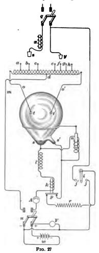
direct current is obtained by placing the plugs z, y in connection with suitable taps a, b, c, d, e, f, g, h along the autotransformer coil; the voltage with these plugs in any position may be further varied somewhat by varying the position of an
