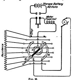
spring d-resistance-switch-battery. The motor is adapted to give three pulling speeds, corresponding to 10, 30, and 40 feet per minute, which can pull an average of 6,000 feet of cable in 6 hours. One charge of the storage battery is sufficient to propel the automobile 20 miles and leave enough current to pull cable the remainder of the working day. The cost of a charge per working day with current supplied at 4 cents per kilowatt-hour is \$1.07.
