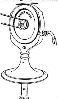
16 inch in diameter on the small sizes of machine, but if sufficient power is not obtained with this size, the nozzle may be drilled to a larger size by an ordinary twist drill.
