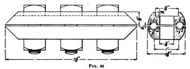
and is now generally required. It should be made of the best quality of malleable iron with high carbon steel bolts. It is usually made to hold a  $\frac{5}{10}$ -inch wire cable.
