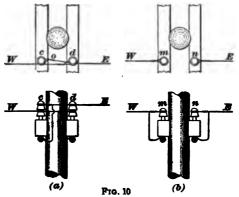
is to use double-groove insulators on both pins and wrap the wire from one direction in the upper grooves of the insulators in figure 8 fashion. The wire from the opposite direction should be wrapped around in the lower grooves in the same manner.
