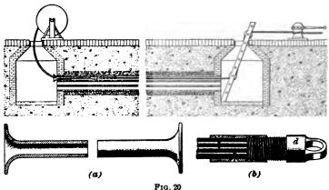
cable grip of iron pipe made to fit the cable snugly. It is fastened to the cable, as shown, by common wood screws, and the piece d to which the drawing-in rope is fastened is screwed into the end of the iron pipe. Better forms of cable grip have been illustrated in Telephone-Line Construction, Part 2.
