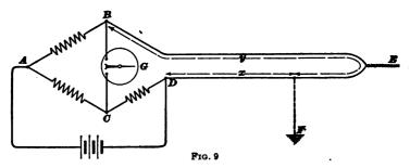
most convenient and best method for locating a ground or cross on a line. The distant ends of the good and bad wires are joined together and the resistance of the loop so formed is measured with the Wheatstone bridge, if not already known from some previous measurement, by connecting as shown in Fig. 9. G is a reflecting galvanometer connected across the arms of a Wheatstone bridge in the ordinary
