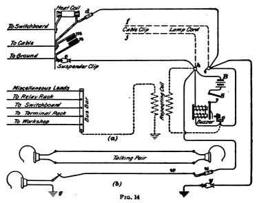
over the cable or line springs, as indicated in the upper part of the figure. A ground between two carbons m, n will cause the buzzer to cease vibrating as the closed circuit h-e-m-n-d-i-e- short-circuits both the buzzer coils and the battery. The ground is removed by taking out and cleaning the carbons.
