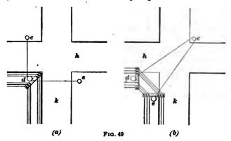
because usually it is unnecessarily expensive. The corner pole should be head-guyed before the line wires are tied. The intersecting streets are h, k, while dc and de in (a) and cd and ce in (b) represent guy wires.
