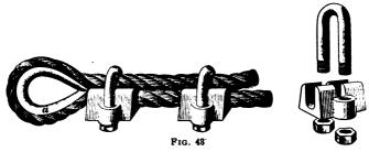
this being made to interlink with that of the anchor rod. Where, however, the guy wire is to be secured to the pole or to a guy stub, the thimble a is not used, but the wire rope is passed twice around the pole as before, and then secured by means of the clamps. Guy wires fastened with clamps can be removed when necessary with no waste of material and much quicker than when twisted together, in the old way, with pliers.
