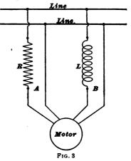
ings are frequently so designed that the necessary phase displacement is caused by the windings themselves, and outside
