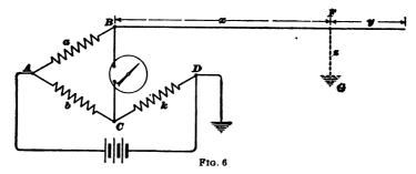
ductivity of the line wire, the distance to the partial ground is obtained. If L is the length of a cable and f the total resistance of the bad wire to the distant end of the cable, the distance to the fault equals  $\frac{x \times L}{f}$ .
