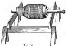
should be provided. These should be from  $\frac{1}{8}$  to  $\frac{3}{8}$  inch wide on the upper edge and from 12 to 18 inches long, depending on the weight and size of the armature to be balanced. They should be set level and parallel, and at such a distance apart that the journals of the armature shaft will rest on them.
