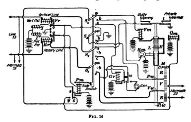
contact z-side switch  $S_{\bullet}$ -contact a-vertical magnet V m-battery-ground. An impulse through the rotary relay R r closes a local circuit through the ground-spring q-private magnet P m-battery-ground.
