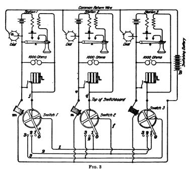
impulses would have been sent through the magnets, and the arm would have moved forwards six steps), thus establishing a circuit from telephone 1 through line wire j-arm e-contact button 2-wires 2-f-line wire q-telephone 2-line wire v-magnets n, m-telephone 1. Thus, the voice currents must pass not only through the telephone instruments, but also through the two magnet coils n, m. They are not strong enough to operate the magnets.
