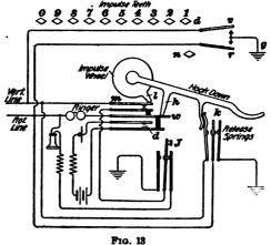
to receive a call. Suppose that the subscriber desires to call 76. He takes down the receiver and puts his finger in hole 7 and pulls the dial around until his finger is stopped by the finger stop. This first opens both line wires
