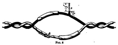
not twisted together. For No. 22 B. & S. wire, the finished joint should include \( \frac{1}{2} \) inch of the insulated wires and 1 inch of the bared and brightened wire.
