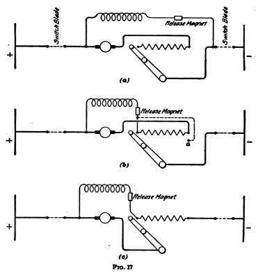
shown in order to make the connections as clear as possible; but such rheostats are now used but little for the following reasons: Suppose that a motor is shut down by opening the main switch and the attendant forgets to move the rheostat arm back to the off-position. When the motor is started up again, the chances are that it will not be noticed that the rheostat
