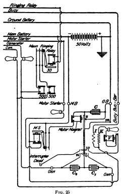
require a regular ringing generator. The main bus-wires may be considered as a continuation of the main bus-wires in Fig. 22 and would replace the transformers, batteries, and all other power apparatus. As pole changers have been fully explained, it will be only necessary to explain the special features of this particular one. The pole changer is normally at restthat is, not in operation. As soon as the shaft of a switch rises one or more steps, the motorstarter circuit is
