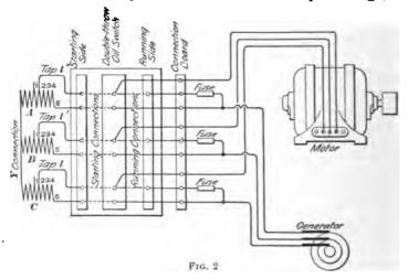
short-circuited, winding, it is generally started by cutting down the voltage applied to the primary. This is usually done by means of an autotransformer inserted between the line and the motor field, the transformer being provided with a double-throw switch, so that it can be cut out when the motor has come up to speed.
