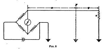
cation of the Blavier, not so convenient as the latter, but suitable when the resistance f of the line is not known with sufficient accuracy for the Blavier method. Besides measuring the resistance b of the line with the distant end open and the resistance c with the distant end grounded, it is necessary to make a third measurement of the resistance d with the distant end grounded through a known resistance o, as shown
