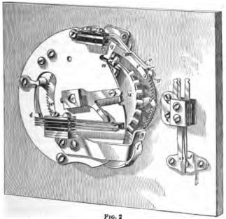
plates is fastened to the door of the telephone box. shaft c extends through the base plates, projecting on both sides. On the front end is mounted a strong clock spring
