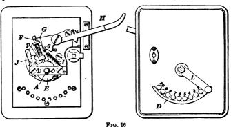
contact always with the one over which it lies. The curved contact piece D is so arranged that the lever will not normally touch it, but, by pressure on the handle of the latter, the two may be brought into electrical contact. H is the usual hook switch. The lever L is mounted on a shaft A passed through the front board of the box, which shaft carries
