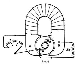
brushes +B and -B, the current in the field coils will be relatively very small compared to the total current as just stated.
