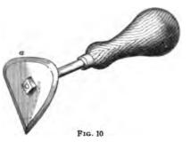
pad being well rubbed with tallow, or with chalk and tallow, to prevent melted solder from sticking to it. A small hand glass or mirror is useful for examining the under side of the joint, and a pair of dividers, or compasses, to make a mark around the cable.
