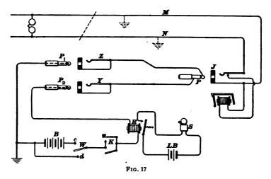
or crossed through a small enough resistance, the relay will be closed when W is placed on c and K is closed.
