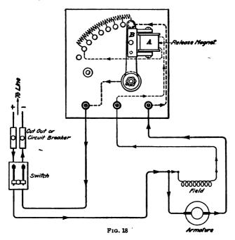
no-voltage, release mechanism so that the rheostat handle will fly to the off-position whenever the power is cut off from the motor.
