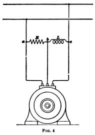
resistance and inductance are rendered unnecessary. In some cases, one of the windings is a main, or working, winding, and the other is used only at starting, being cut out by open-circuiting it by means of a switch after the motor has attained its speed.
