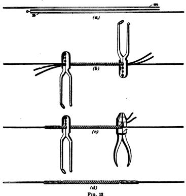
turn at each end would hold, if soldered, while the wire of which it was made would break. Hence, the proper soldering of an iron-wire joint increases its strength as well as its conductivity.
