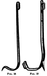
spur, and therefore is secured to the outside of the leg. In the Eastern pattern, the rod is on the same side as the spur, and is therefore secured to the inside of the leg.
