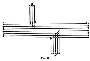
▼ splices are never made in rubber cables, because they are not made large enough to warrant such treatment, and because their nature of construction is such that weather-tight splices of this sort could not be made. This practice is resorted to only in the case of lead-covered cables.
