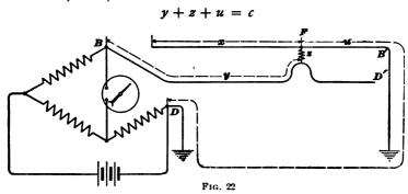
Subtracting the last equation from the sum of the first two and then solving for the resistance x from the testing station to the fault gives the following formula:
