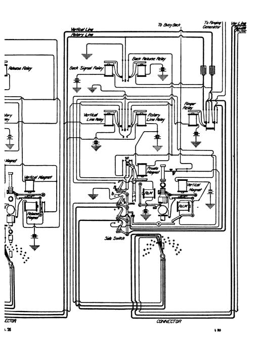
line is shifted by the line switching relay from the vertical relay of this first selector to the vertical wiper and vertical trunk line running to the second selector.
