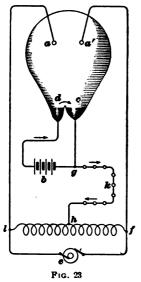
the negative impulse of an alternating current can be made to flow in the same direction as the positive impulse; in other words, the alternating current is rectified and the entire current used. The tube has four electrodes; d is an auxiliary anode through which current enters the tube from a battery b, c the cathode, and a, a' the anodes to which the wires from the dynamo e or a transformer are connected.
