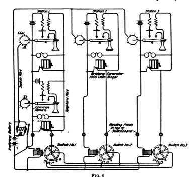
calling subscriber should turn his dial to the black space, that is, back to its normal position; otherwise, the two stations left connected together would both be rung up the next time a third party called either station. There seems to be no provision in this system to prevent a subscriber from securing connection with a line that is busy.
