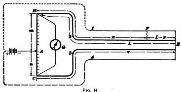
regular Wheatstone bridge, thereby simplifying the test. In Fig. 14, BC represents a slide wire, which may be a piece of No. 24 B. & S. German-silver or iron wire stretched between posts BC so as to be over a scale divided into exactly 1,000 equal divisions, preferably millimeters. The smoother and more uniform the diameter and material of the wire BC, the
