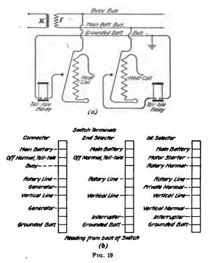
selector to its normal position. The release magnet of the connector is connected from the main-battery bus through springs t', v to the grounded-battery bus, thereby restoring the connector to its normal position. If the receiver at the called telephone is hung up first, the switches are not released.
