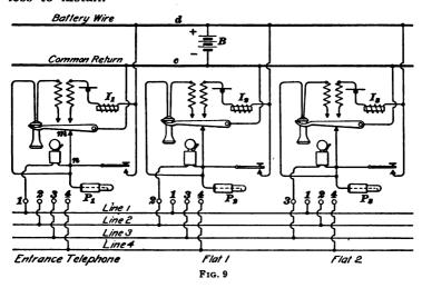
17. Apartment-House System.—In Fig. 9 is shown a similar arrangement that is more suitable for communication between the vestibule and the various flats in a modern apartment house because it is unnecessary to return the plug to its home jack or to remove it from any jack in order for
