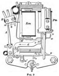
block of contacts B. first position a is the normal position on which the arms rest when the switch is released; b is the position held while selecting a line; c is the final position. This side switch is under the tension of a spiral spring a', shown in Figs. 6, 8, and 9, that tends to make it rotate about the axis b'b'. It is restored to its normal position on the row of contacts a, Fig. 9, by the action of the armature W of the release magnet Qm, Fig. 6,
