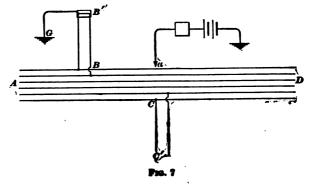
prefer a receiver for this test in place of the buzzer, and claim that the office end of the cable should be connected up first and all testing done from there.
