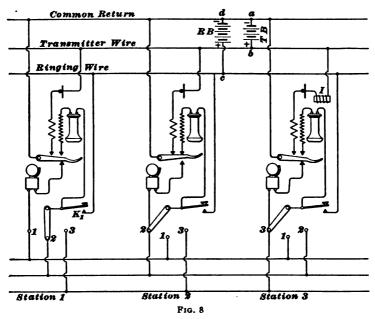
wires are required than there are stations. The necessary number of cells may be connected between b and c in series with TB and all the cells between a and c used as a ringing battery.
