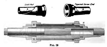
Fig. 29 shows the novelty slidable sleeves that are used for making an ordinary straight joint between two cables. It consists of a brass shell with hubs a, b tinned ready for soldering, and screwed on each end. To make a joint, unscrew the tapered screwed end a, pass it over the cable, and slip the rest of the sleeve on the opposite end of the cable.
