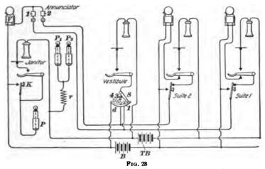
button K for ringing, through plug P and the proper jack, the bell in any apartment. Each suite is provided with a telephone, bell, and push button; by means of the latter the annunciator and bell in the janitor's apartment may be operated.
