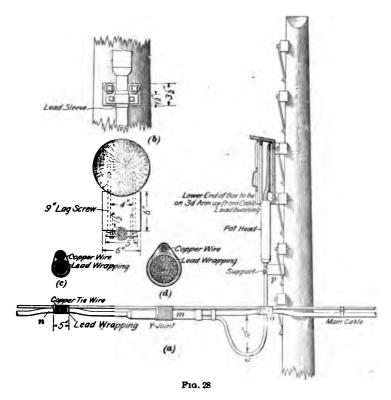
9 feet long and then spliced to the main cable by a  $\forall$  joint. The pothead should be securely fastened to the pole at p, which is just below the wiped joint, by means of wooden blocks and iron straps, the cable being protected where the strap presses on it by a piece of sheet lead wrapped around the cable to form a sleeve. At (b) are shown two views on a larger scale of the details of the cable support at p.
