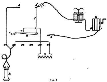
the inspector would at once conclude that the signaling apparatus and circuits were all right, and that the fault was somewhere in the talking apparatus or circuits. Furthermore, from the fact that the instrument would not receive speech, he would know that the fault was not in the primary circuit because that circuit has nothing whatever to do with the receiving
