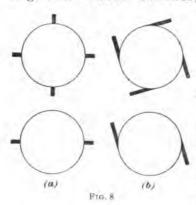
toward the center of the commutator. Tangential brushes, Fig. 8 (b), frequently made of copper, are found, as a rule, only on low-voltage high-current machines. Radial brushes are nearly always made of carbon and are always used on machines designed to rotate in either direction. The brushes should be so placed that with a slight end
