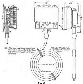
diameter of .84 inch. All threaded joints are made tight by coating the threads with white lead as they are put together. The brass screws b are known as No. 8, 32,  $1\frac{1}{4}$ " machine screws and are provided with brass or copper washers.
