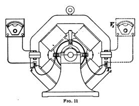
than this, the windings should be examined separately, the ground located, and, if possible, removed. Before making this ground test on a railway or other permanently grounded dynamo, the grounded terminal should be disconnected from the circuit.
