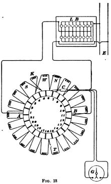
obtained on the lower side, except when bars 15 and 16 are bridged. There will then be a violent throw of the needle, because the voltmeter will be connected to A and B through the intervening coils. The break is thus located in coil T. As a temporary remedy for this, bars 15 and 16 may be connected together by a jumper or piece of short wire. The defective coil T should, however, be repaired as soon as possible.
