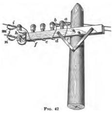
or with half sleeves. The bridle wires are held under the crossarm with wooden cleats c, d, e, f. The drop line is deadended by means of sleeves i, j around the glass insulators on a so-called universal two-insulator iron h, which is fastened to the arm with two \frac{2}{8}-inch carriage bolts. To the pro-
