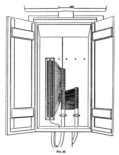
arresters is shown in Fig. 31. Pole boxes are intended to be waterproof, but sometimes they are not, and, hence, special care should be taken to make the cable heads moisture-proof.
