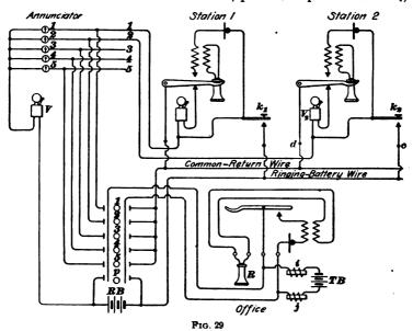
which will operate the annunciator 1 and bell V in the office. The office attendant pushes in the corresponding button 1 on the automatic switch, restores the annunciator, takes down his receiver, and attends to the call.
