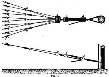
insulators. Hard-drawn copper wire stretches considerably and allowance should be made for the proper sag in the middle of the loop as given in Table XII or Table XIII. In about 8 months after the line has been finished, the wire will have reached its maximum sag; then, the slack should be taken up. From that time on, there may be a very little sag, but, at the end of 2 years, the wire will have practically ceased stretching, and will require no further attention.
