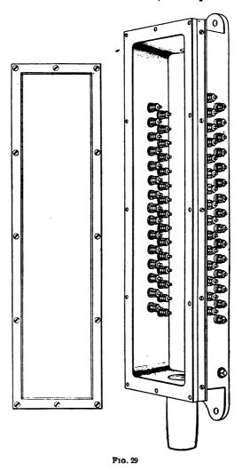
insulating bushings c to the outside of the box. In a cable head of this style, it is necessary to solder the wires to the terminals.
