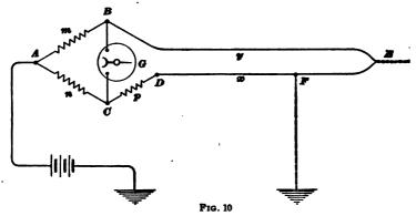
E to F, x the resistance from D to F, and R, the total resistance of the loop, is equal to x + y. Then, when the bridge is balanced,  $\frac{m}{n} = \frac{y}{p+x} = \frac{R-x}{p+x}$ ; mp + mx = nR - nx; mx + nx = nR - mp. Hence, the resistance,  $x = \frac{nR - mp}{m+n}$
