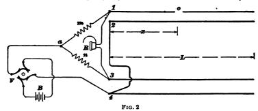
The conductor 1 is open at o, while its mate 2 and the pair 3, 4 are supposed to be good wires; m, n represents two adjustable arms of a Wheatstone or slide-wire bridge and R a telephone receiver. The connections are made, as here shown, at one end of the cable and the resistance in the arms m, n adjusted until no sound, or a minimum sound, is produced in the receiver R. Then the distance to the fault o is given by the formula:
