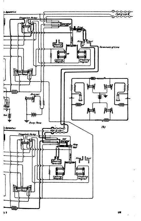
held in its advanced position by the sluggish locking magnet, which will not respond to the slight disturbances of the selecting relay that sometimes occur during revertive ringing. The selector brushes are now in contact with the terminals of the desired line and the circuit, as shown in Fig. 7, is ready for signaling.
