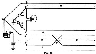
success, according to Adolph Jameston in The American Telephone Journal, by the following method: In Fig. 13, w is a pair of wires in good condition the full length of the cable and s is the split pair being tested, the conductor s of which is connected with one wire s of the other split
