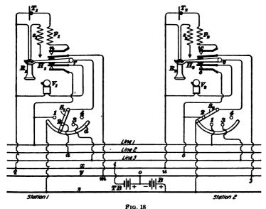
the primary circuits are closed in the ordinary manner. secondary or talking circuit may be traced from the secondary winding S at station 4 through the receiver R to the common talking wire, thence through the receiver R and secondary S at station 1 to the hook lever H, and thence by wire 1 to station 4 and through button 1, switch lever L, switch hook H, and back to the secondary coil at station 4.
