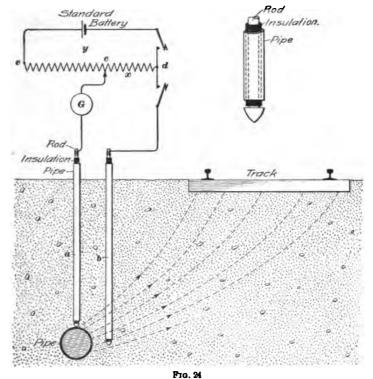
would disturb the normal current flowing between the pipe and ground, but by balancing the unknown electromotive force against a known electromotive force from a standard battery. The resistance cd is adjusted until the galvanometer G indicates zero current, an the electromotive force between the pipe and ground then bears the same relation to the known electromotive force of the standard battery that
