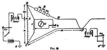
which BC represents a slide-wire bridge; R, a known resistance; G, a sensitive galvanometer with its usual shunt r and short-circuiting key k; CFg', the wire in use; and HF, the line wire, which is crossed at F with the other line wire and is open beyond the cross. To make the test, set the slide about midway along the slide wire BC, short-circuit or remove all the resistance at R, open the galvanometer short-circuit key k, and adjust the position of A along the slide wire until
