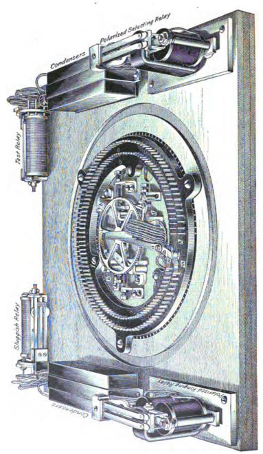
by the locking magnet e with its pawl f. These magnets are of the common double-coil type, their armatures being softiron levers, on the ends of which are mounted the pawls engaging the ratchet-wheel teeth. The leverage of the selecting-magnet armature is such as to make it quick-acting, while that of the locking magnet makes its action more sluggish. The action of the locking magnet is made
