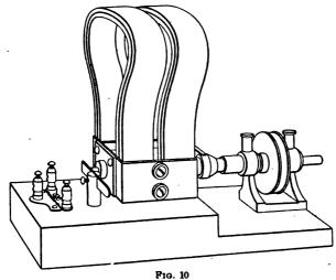
substations. The only essential difference in the types is in the application of the driving power. The frequency of the machine must be that best suited to the natural vibration frequency of the ringers used in the telephone instruments, the most common frequency being in the neighborhood of  $\cdot$  20 cycles per second, corresponding to from 2,200 to 2,400 alternations per minute.
