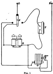
across the circuit, and may be used as either a transmitter or a receiver in communicating with another party on the line. When the generator is at rest and the switch is thrown to the right, the telephone T alone is connected in the circuit between the binding posts, the generator being shunted out of circuit by the automatic shunting device. If, however, the generator should be operated while the switch is in this position, the current from it will pass
