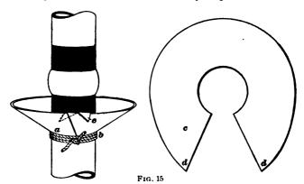
should then be attached temporarily to the cable directly under the joint so as to catch the solder and raise the
