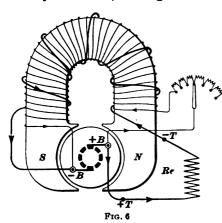
tial at the terminals of the machine is not automatic; it is accomplished by a mechanical movement of an arm or contact. This movement of the rheostat arm is sometimes imparted automatically by a magnet controlled by the current in the external circuit. But, more often, when a very constant potential is
