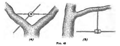
Fig. 43 will hold the wire securely and yet allow sufficient play to preserve them from breaking under the strain caused by the swaying of the trees. No wires should be attached to trees unless it cannot be well avoided.
