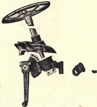
Fig. 26. Worm and Sector Type of Steering Gear. Corbin Motor Vehicle Corporation, New Britain, Conn.
