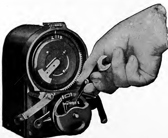
FIG. 223.—Eisemann magneto, type G4, I Edition, with distributor removed showing setting marks for timing, also method of adjusting interrupter contacts.
