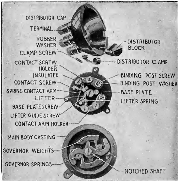
FIG. 95.—Construction of Atwater-Kent ignition unit, type K-2.
