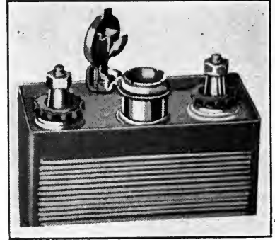
FIG. 36.—Top of Edison storage cell showing filling aperture open for adding water.
