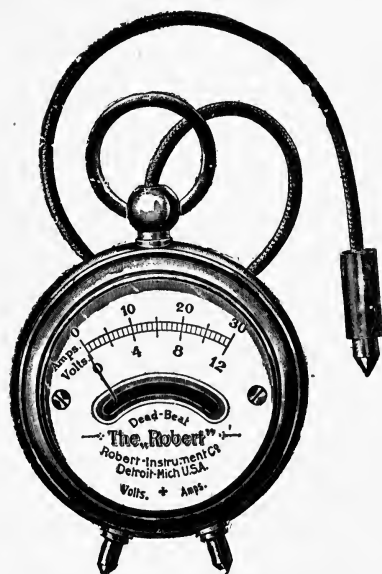
FIG. 28.—Typical pocket volt-ammeter for testing dry cells.
