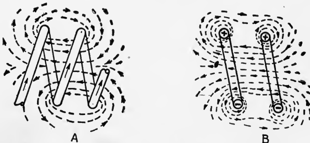
FIG. 18.—Magnetic lines of force around two adjoining loops carrying current in the same direction.
