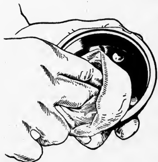
FIG. 92.—Method of cleaning distributor head.
