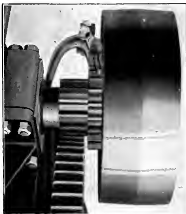
No. 1 Top View—shows low speed pinion in mesh with compensating gear for traveling ahead.
