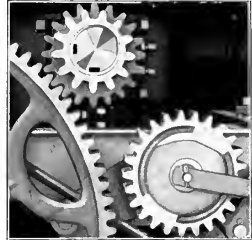
No. 3 Side View—shows high speed pinion shifted over in mesh with compensating gear for traveling ahead.
