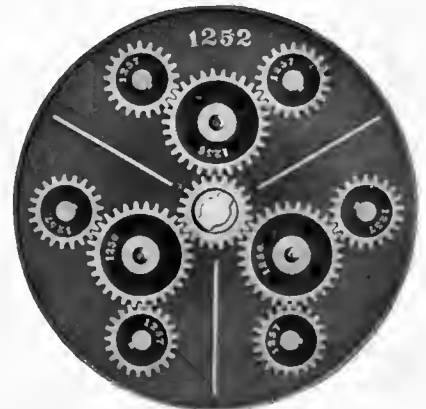
End View of I. X. L. Separating Device Showing Arrangement of the Gearing.
