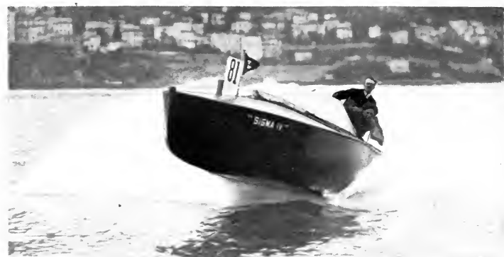
The Henry Farman hydro-biplane, about to rise and about to alight. Below is a fast flat-bottomed motor-boat, showing how the bows rise from the water at high speed.
