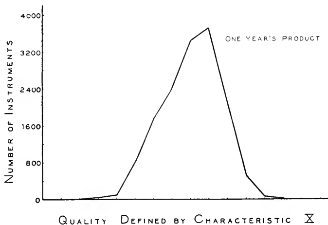
Fig. 1—Polygon showing distribution in quality for 15,050 units of product. Do these data present any evidence of lack of control?
