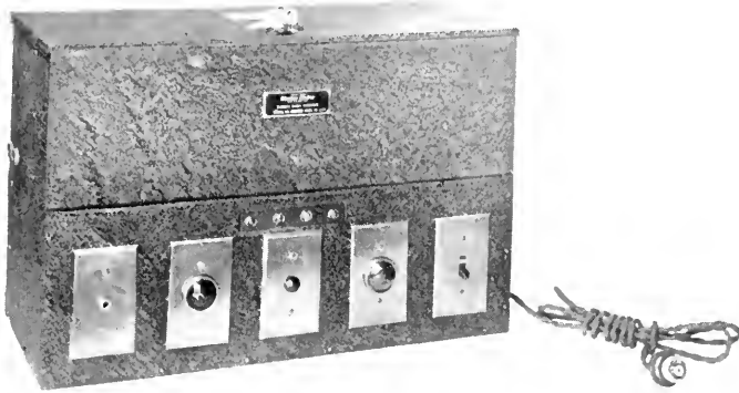
Fig. 3—Exterior view of receiving set. (The external appearance of the A.C. and D.C. models is the same)
