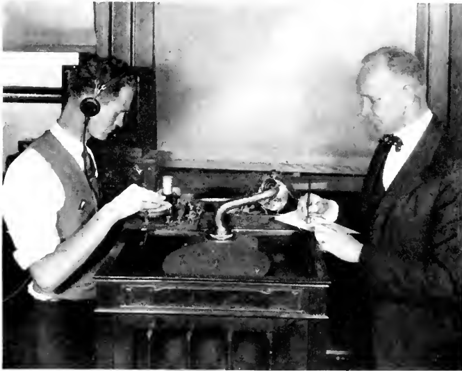
Fig. 21—Bridge for measuring mechanical impedance, being used for determining the impedance of a phonograph horn
