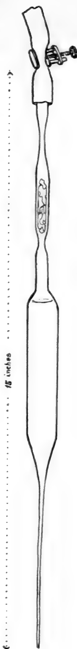
FIG. 19.—Roux's tube for liquid cultivation in vacuo .
