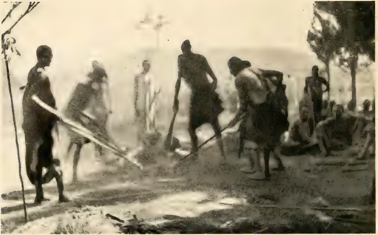
Levering smelted iron from the furnace with tree branches
