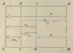
represent the chamber of the gun, which we will suppose filled with powder without compression, and further that one pound of the powder fills a space of 27.68 cubic inches. The gravimetric density and density of loading are each unity; and if  $v_1$  is the volume of the chamber, it follows that
