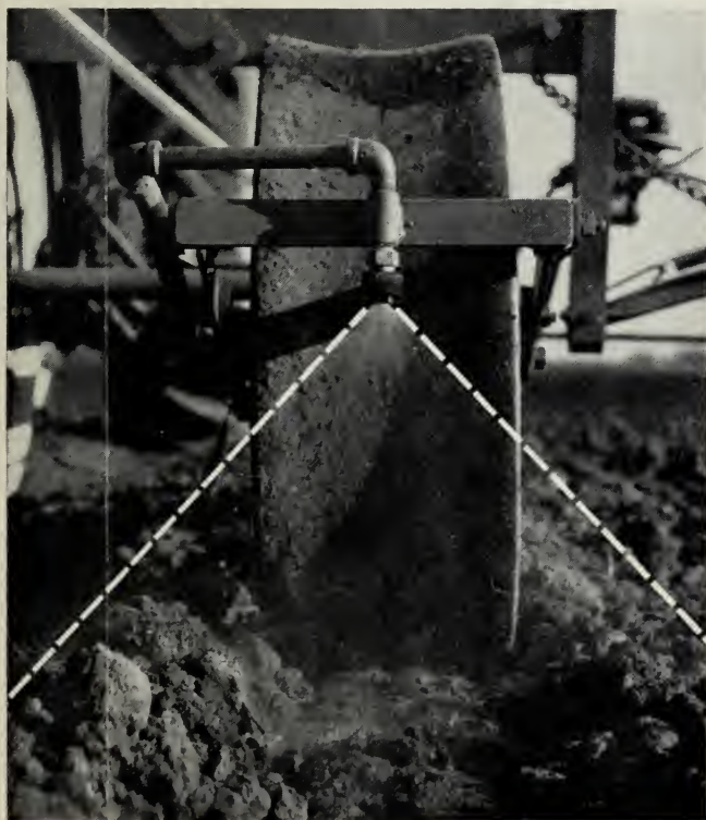
Sprayed band should extend beyond the press-wheel ridges. (Fig. 2)
