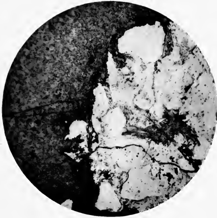
FIG. 1.—Tourmaline, in felted mass of fine needles, replacing quartzite at margin of tourmaline vein. A cluster of tourmaline needles is seen within the quartzite. Cræsus Gold Mine. Ordinary light ; diam. \times 28 .
