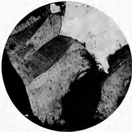
FIG. 3.—Relatively coarse crystalline aggregate of chlorite, showing the basal cleavage and replacing quartz. The dark mineral is pyrite. Polarised light ; diam. \times 66 .
