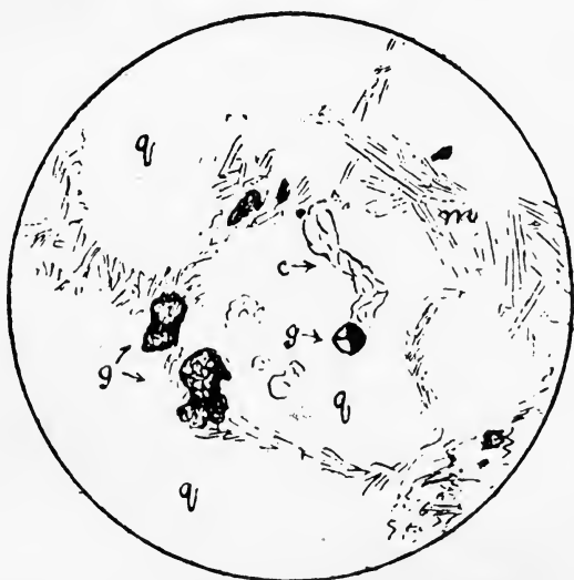
FIG. 1.—Crystal of Gold (octahedral faces predominant) within quartz grain in the matrix of banket: g =gold, q =quartz, c =chlorite, m =muscovite. Diam. \times 200 .
