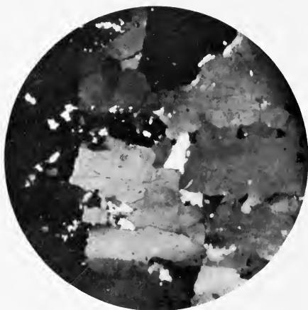
FIG. 2.—Portion of a vein-quartz pebble, showing fracturing of a somewhat different character. Small individuals of clear recrystallised quartz are to be seen here and there.
