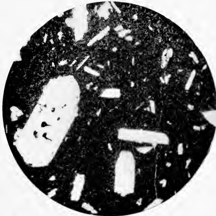
FIG. 3.—Enstatite andesite. The large crystal to the left is composed of uralite. The others are mostly plagioclase feldspars. Blue Sky Gold Mine. Ordinary light ; diam. \times 28 .
