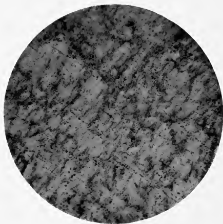
FIG. 2.—Portion of a black vein-quartz pebble, showing innumerable minute inclusions arranged in two superimposed systems, one forming an irregular mesh-work, while the other runs in straight lines across the section. Ordinary light ; diam. \times 71 .
