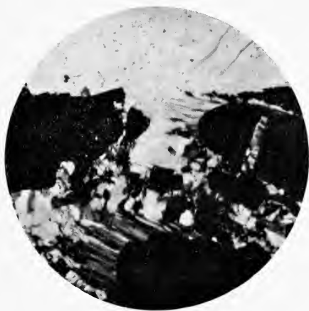
FIG. 1.—Fibrous quartz at the acute ends of two pyritic nodules. The same substance fills a crack in the upper nodule. Nicols crossed; diam. \times 15 .
