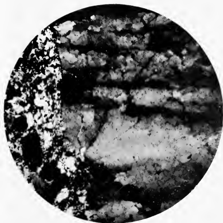
FIG. 1.—Marginal portion of a vein-quartz pebble, showing strain shadows, fracturing, and innumerable minute inclusions. To the left appears some of the matrix of the banket.
