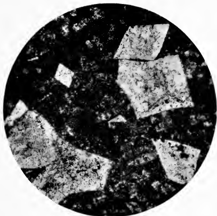
FIG. 1.—Much altered porphyritic igneous rock composed of a very fine aggregate of quartz, chlorite, leucoxene, etc., and conspicuous crystals of dolomite. With higher magnification the structure of the groundmass can still be seen, even within the dolomite rhombs. Randfontein Central Gold Mine. Ordinary light ; diam. \times 17 .
