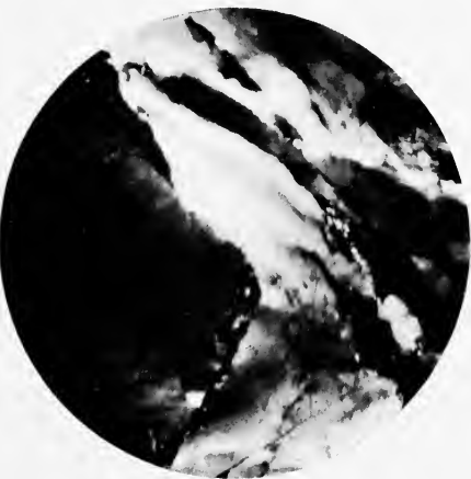
FIG. 3.—Portion of indented contact of two vein-quartz pebbles. Note the strain shadows. The pebble on the left is partly replaced by sericite at the contact. Nicols crossed ; diam. \times 15 .
