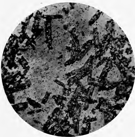
FIG. 1.—Portion of chloritoid-schist pebble. The matrix is mainly a fine-grained quartz mosaic. Ordinary light ; diam. \times 22 .
