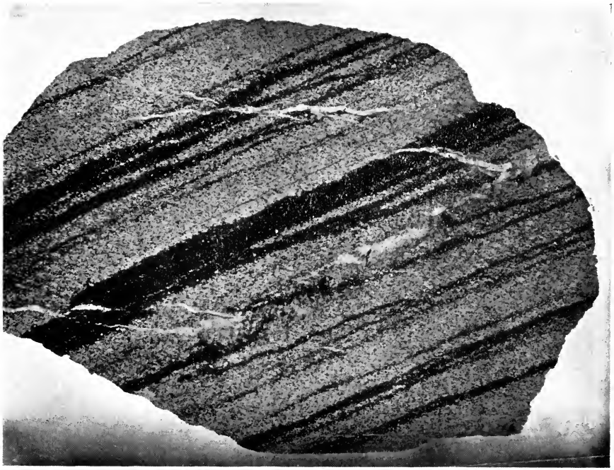
FIG. 1.—Large-sized thin section of banded pyritic quartzite, photographed by transmitted light. The dark bands are pyrite. Meyer and Charlton Gold Mine. Diam. \times \frac{3}{4} .
