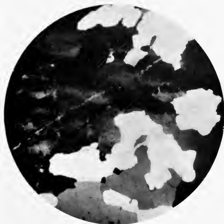
FIGS. 3 and 4.—Portions of the same pebble as in Fig. 1, showing different degrees of recrystallisation. The recrystallised quartz is unstrained and free from inclusions.
