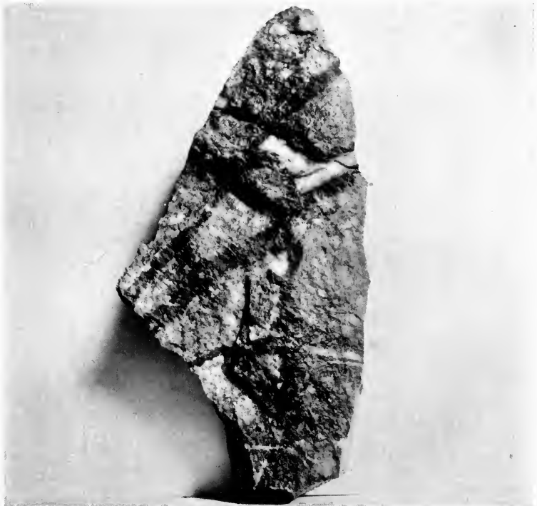
FIG. 2.—Pebbly quartzite, traversed by veinlets of tourmaline, from the Robinson Deep Gold Mine. Diam. \times \frac{1}{3} .
