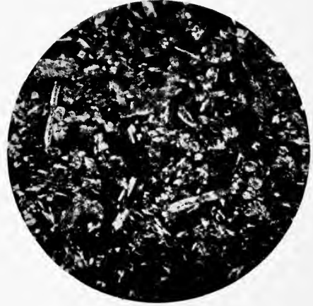
FIG. 4.—Much altered igneous rock, now consisting of quartz, chlorite, calcite, and leucoxene. The original structure is preserved. Randfontein Central Gold Mine. Ordinary light ; diam. \times 15 .
