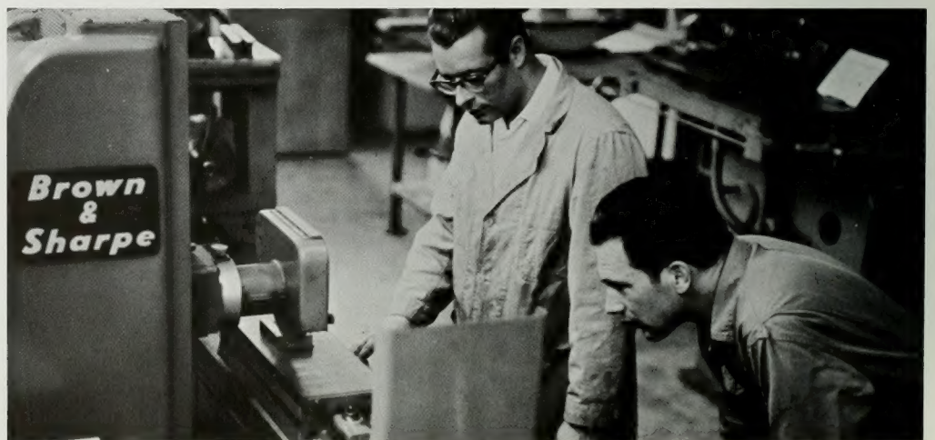
Students in Tool and Manufacturing Technology (right) use a surface grinder to put fine finish on metal surface.
