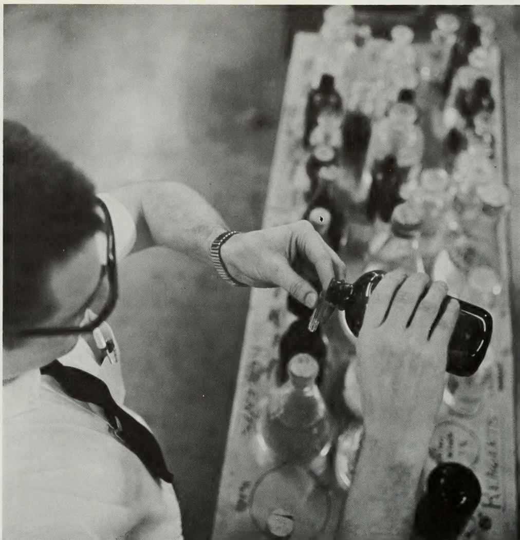
Student looks for a silver mirror when making Tollen's reagent test for reducing sugar.
