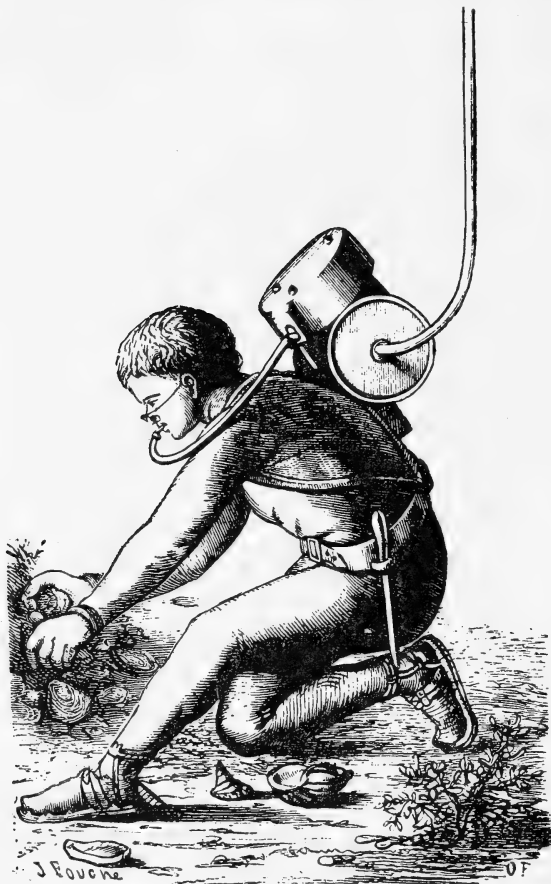
Fig. 8—Diver equipped with the Denayrouze regulator, helmet removed.
