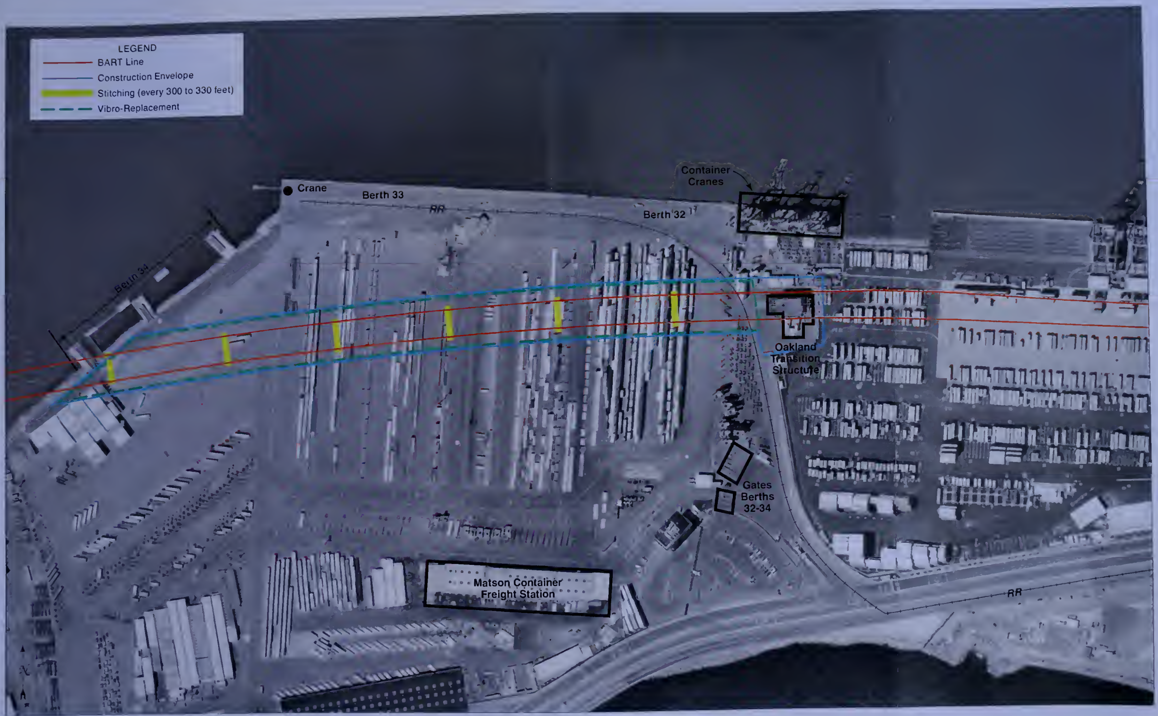
Figure 2-7. Aerial Detail of Stitching the Tube and Vibro-Replacement at the Oakland End
