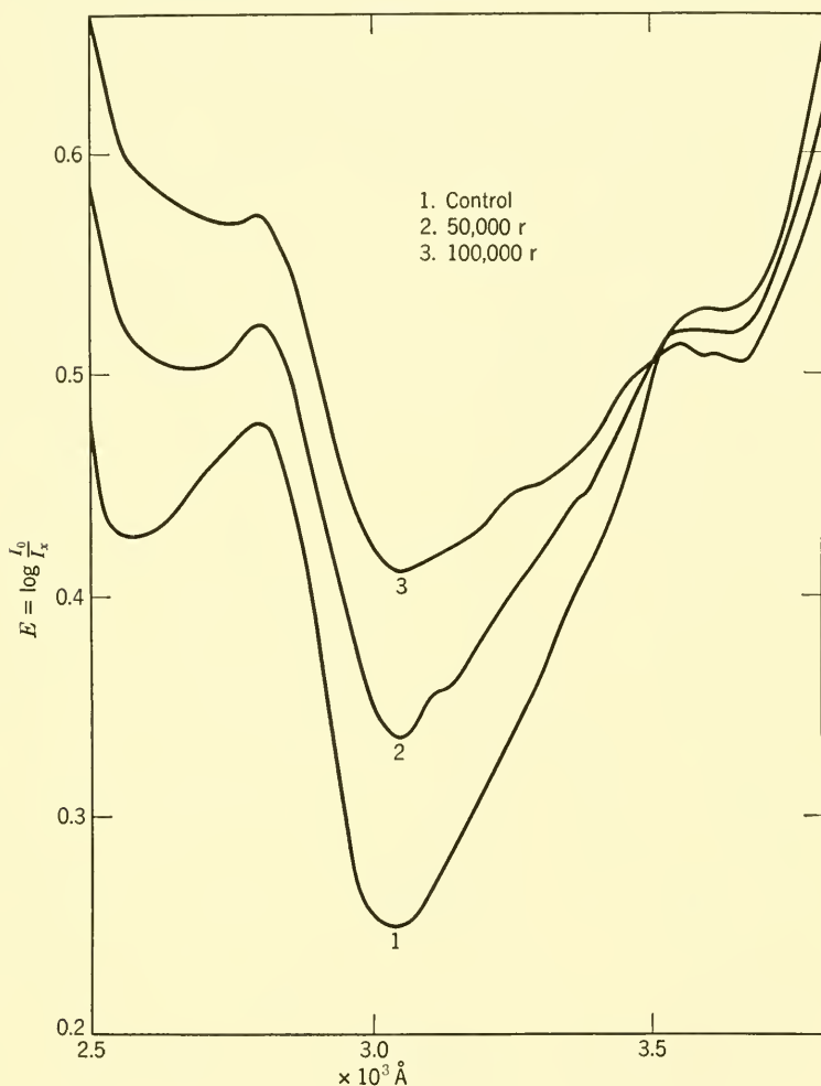
FIG. 4. Effect of x-ray irradiation on the protein moiety of ferricytochrome c, dissolved in 0.005 M phosphate buffer, pH 7.72. Abscissa : Wavelength in angstrom units; ordinate : optical density E .
