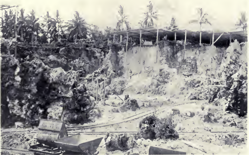
Ocean Island Phosphate Workings. Foreground: Most of the phosphate has been removed exposing the coral limestone pinnacles. Background: Phosphate deposit is intact and exists mostly in the form of gravel with occasional large boulders of phosphate rock.
