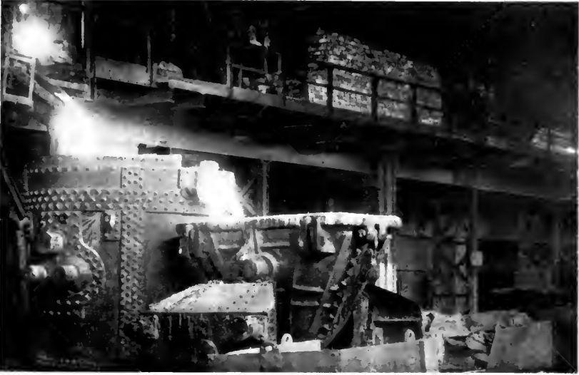
Pouring Slag and Metal from Basic Open Hearth Furnace. The molten slag is seen overflowing from the steel ladle into the slag ladle.
