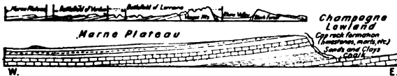
FIG. 58—Ideal east-west cross-section of the Marne plateau, showing how different layers of the cap rock come to the surface in this direction, thereby varying the terrain of the battlefield. The key shows the relation of this cross-section to the cross-sections of the Battlefields of Verdun (Fig. 78) and Lorraine (Fig. 99) and forms a continuous section from the Marne plateau to the Black Forest.
