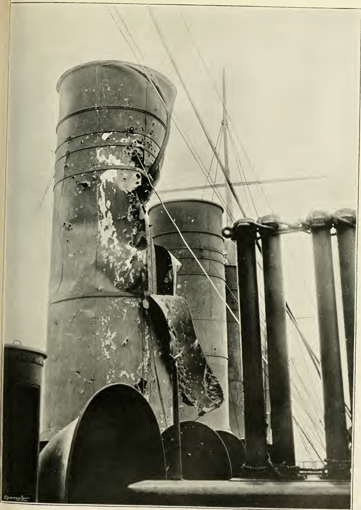
DAMAGE TO THE SECOND FUNNEL ON BOARD THE CRUISER "GROMOBOI" (PORT SIDE).
