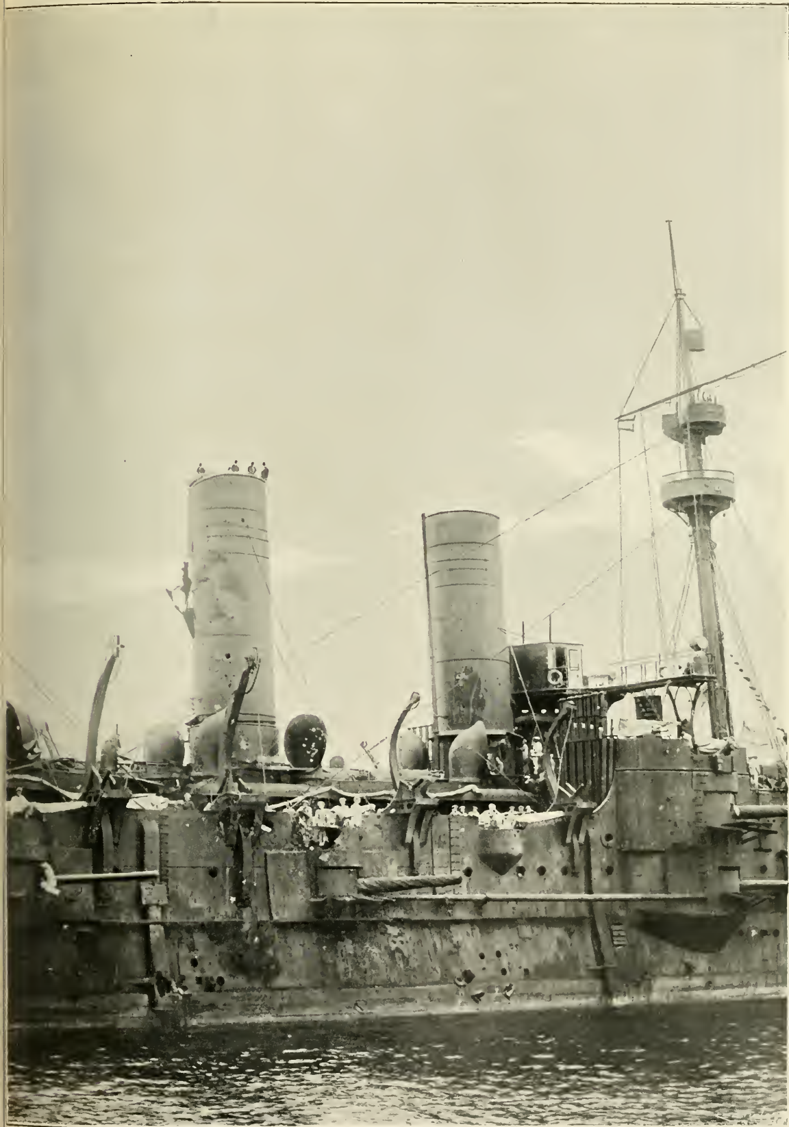
GENERAL VIEW OF DAMAGE TO THE STARBOARD SIDE OF THE CRUISER "GROMOBOL."
