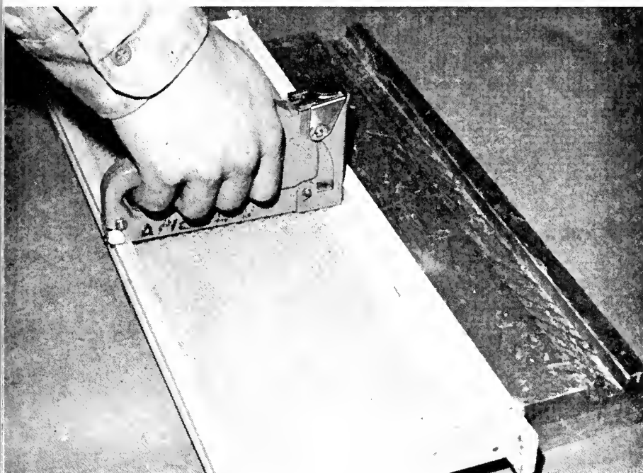
Using a compression stapler to fasten plastic-base foundation in a shallow frame.
