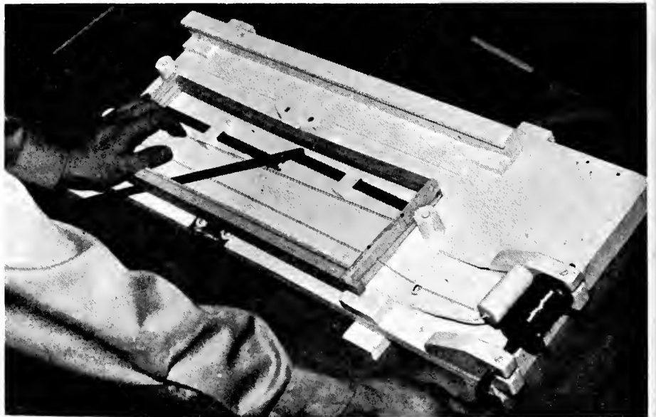
Wiring frames in a homemade wiring device. A deep frame compressed with a metal clamp is shown in the illustration at the top. A shallow frame compressed against a wooden stop is shown at the bottom. (Fig. 17)
