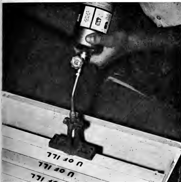
A branding iron and propane torch used to identify frames and other wooden equipment. (Fig. 64)
