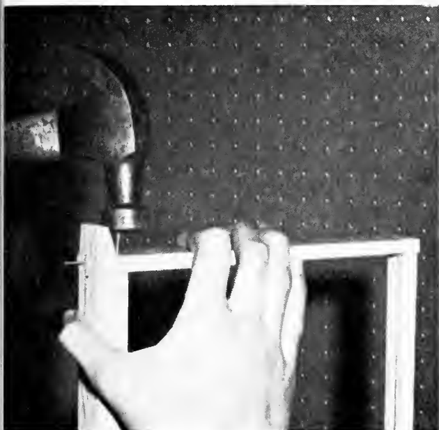
Cross-nailing the end and top bars of the frames.
